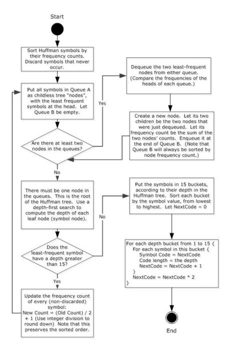
Figure 2: Length-limited canonical Huffman code construction method.
