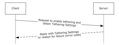
Figure 1: Tethering Control Channel Protocol request-reply sequence
