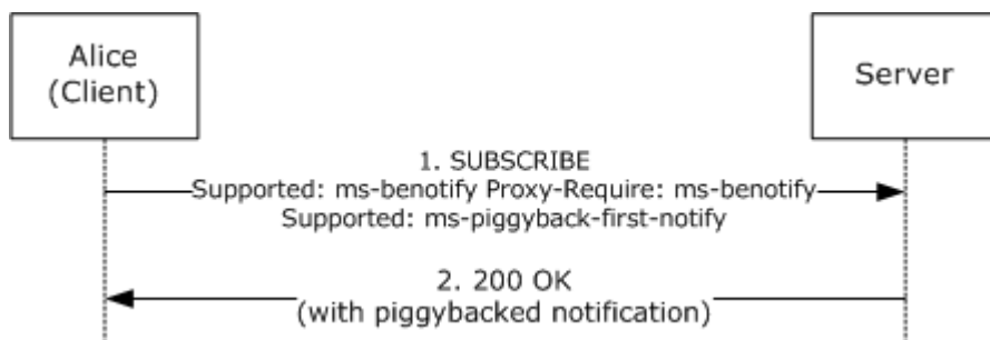
Figure 3: Batched SUBSCRIBE request and piggybacked NOTIFY example
