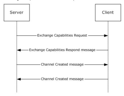
Figure 2: Channel setup sequence
