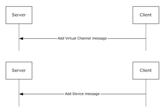
Figure 3: New device sequence
