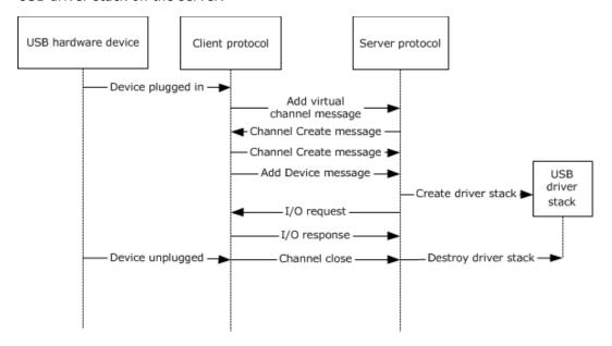
Figure 1: USB stack flow
