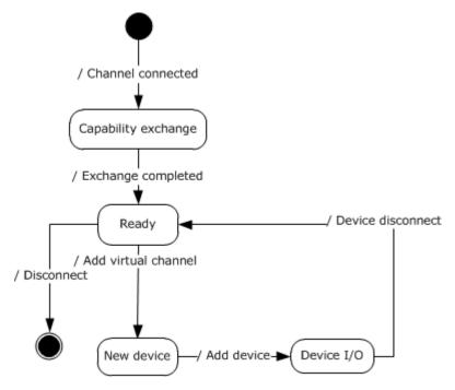
Figure 5: Client and server state transitions
