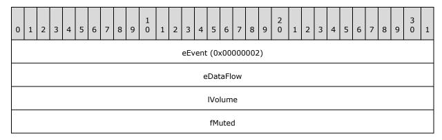
**eEvent(4 bytes):** A 32-bit unsigned integer that specifies message type. The value for SAE\_VolumeChange is 0x00000002.
