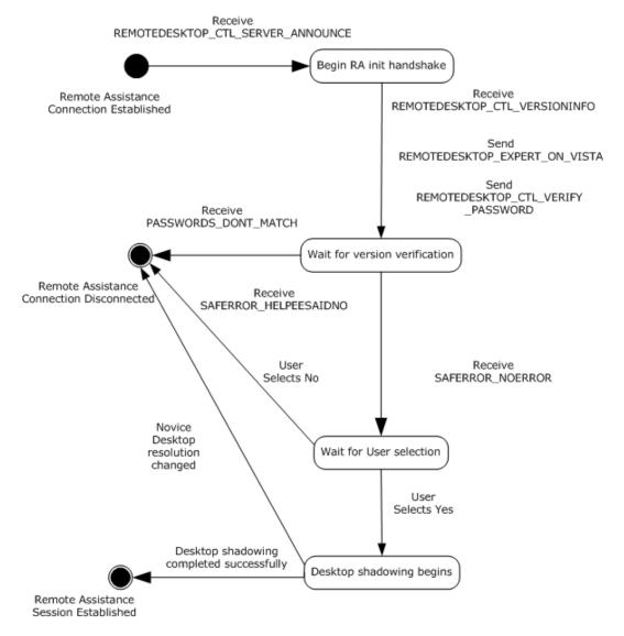
Figure 4: Remote Assistance session initialization version 2 state diagram (from the expert/client perspective)
