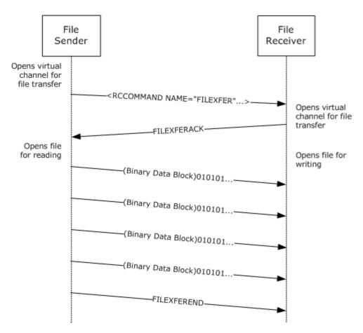
Figure 11: File transfer packet sequencing
