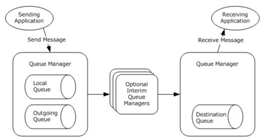
Figure 6: Message Queuing System deployed over a network
