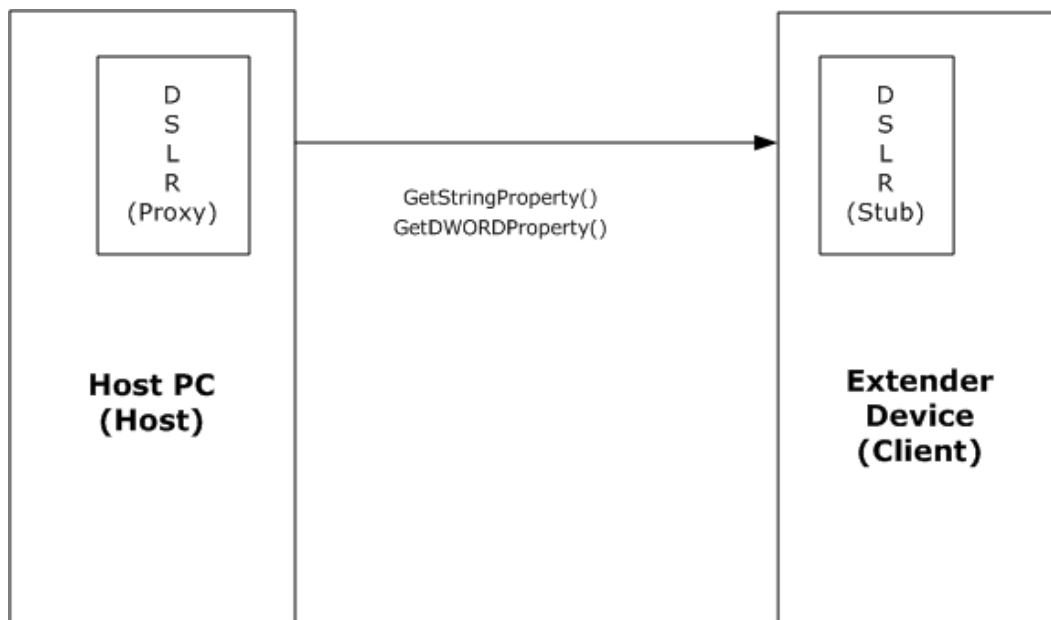
Figure 1: Device Session Property Access Protocol block diagram
