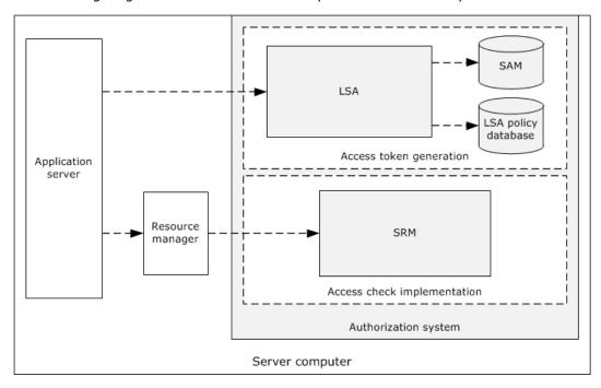
Figure 9: Internal components of the DAC system
