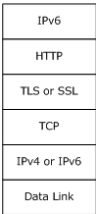
Figure 3: IP-HTTPS server protocol stack when using HTTPS encapsulation
