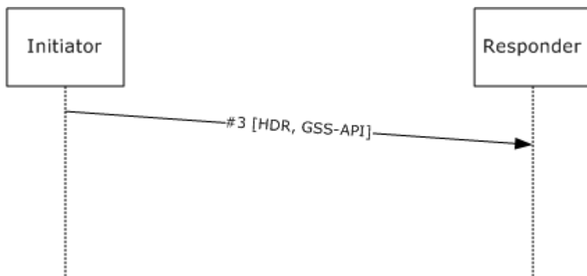
Figure 28: GSS-API initial exchange packet
