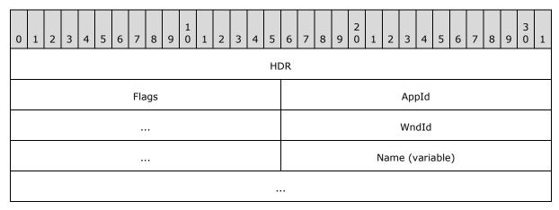
**HDR (4 bytes):** The common PDU header (as specified in section 2.2.1). The **Type** field of the common PDU header MUST be set to ODTYPE\_WND\_CREATED (0x0005).
