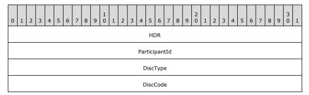
**HDR (4 bytes):** The common PDU header (as specified in <u>Common Order Header (section 2.2.1)</u>). The **Type** field of the common PDU header MUST be set to ODTYPE\_PARTICIPANT\_REMOVED (0x0007).
