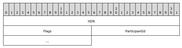
**HDR (4 bytes):** The common PDU header (as specified in <u>Common Order Header (section 2.2.1)</u>). The **Type** field of the common PDU header MUST be set to ODTYPE\_PARTICIPANT\_CTRL\_CHANGE (0x0009).
