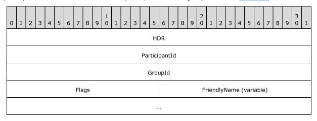
**HDR (4 bytes):** The common PDU header (as specified in <u>Common Order Header (section 2.2.1)</u>). The **Type** field of the common PDU header MUST be set to ODTYPE\_PARTICIPANT\_CREATED (0x0008).
