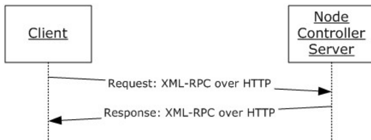
Figure 1: Client-server message exchange
