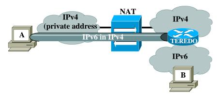
• Teredo uses a specific prefix. The address includes the IPv4 and port number of the host.
