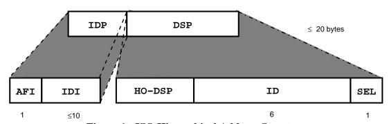
Figure 1 - ISO Hierarchical Address Structure
