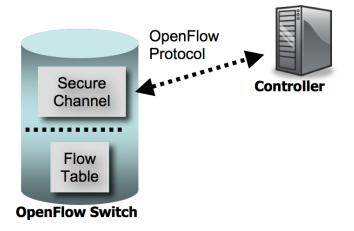
Figure 1: An OpenFlow switch communicates with a controller over a secure connection using the OpenFlow protocol.
