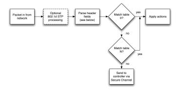
Figure 2: Packet flow in an OpenFlow switch. As discussed in Section 4.5, support for 802.1D is optional.
