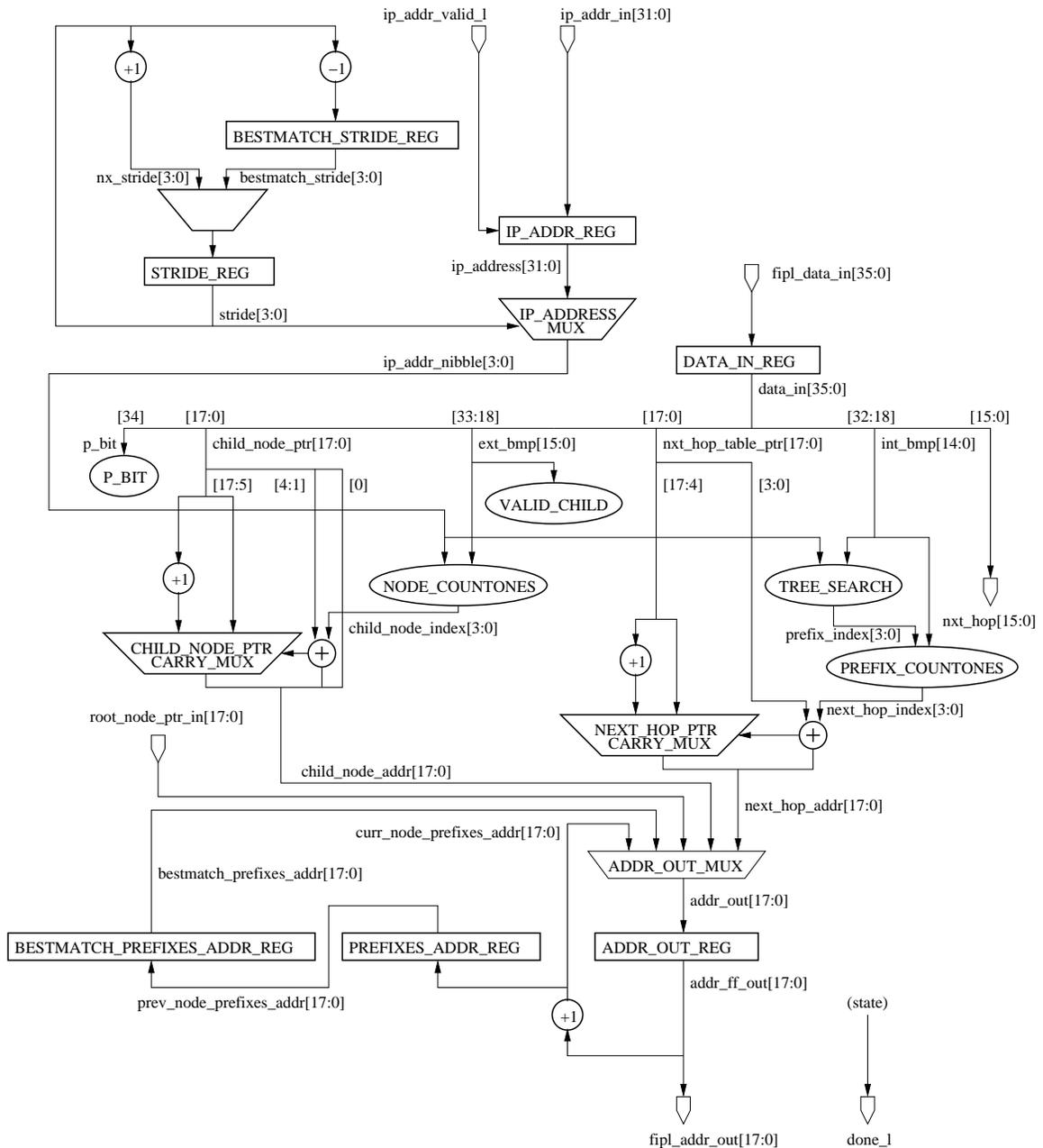
Figure 3.8: FIPL engine dataflow; multi-cycle path from input data flops to output address flops can be scaled according to target device speed; all multiplexor select lines and flip-flop enables implicitly driven by finite-state machine outputs.
