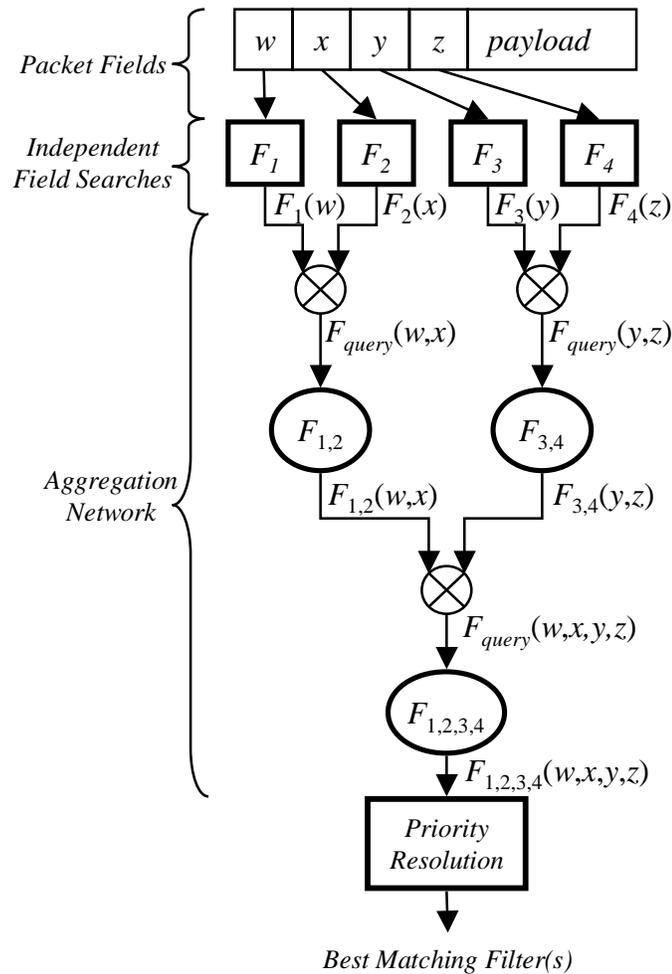
Figure 7.1: Example configuration of *Distributed Crossproducting of Field Labels (DCFL)*; field search engines operate in parallel and may be locally optimized; aggregation nodes also operate in parallel; aggregation network may be constructed in a variety of ways.
