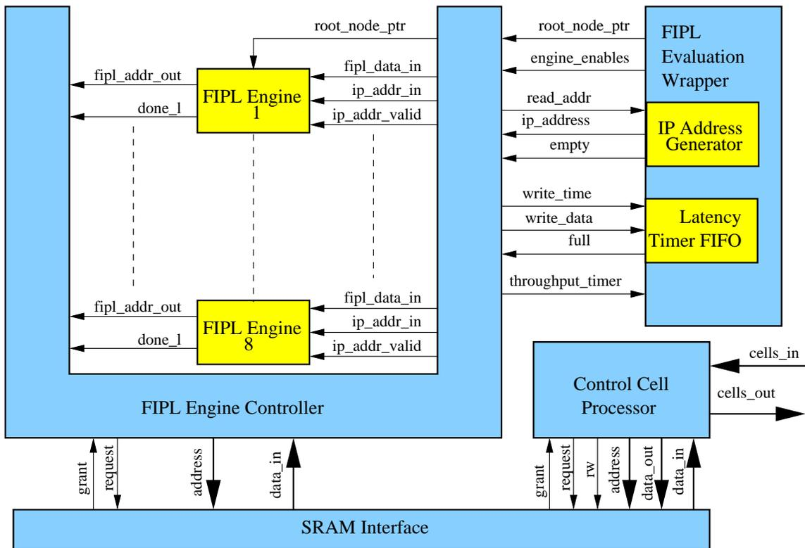
Figure 3.13: Block diagram of FIPL evaluation environment.
