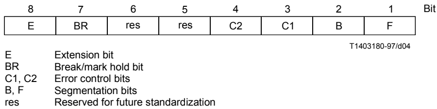
FIGURE 4/V.120 Header octet format
