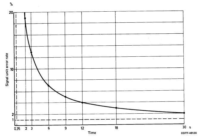
Consecutive signal units received in error for 350 ms will initiate changeover. Note – The curve is based on a uniform distribution of errors.
