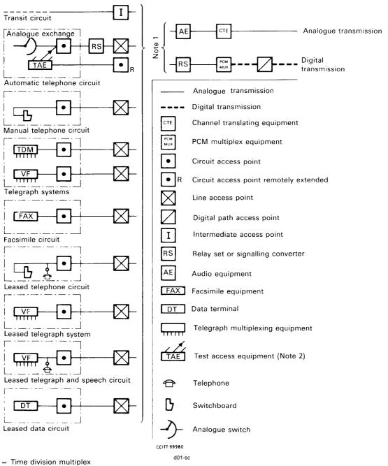
TDM = Time division multiplex VF = Voice frequency multiplex
