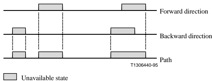
Figure A.2/G.826 – Example of the unavailable state of a path
