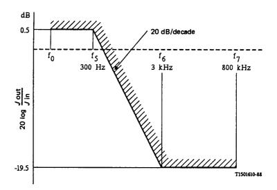
Note I - The frequency  $f_0$  should be less than 20 Hz and as low as possible (e.g. 10 Hz), taking into amount the limitations of measuring equipment.
