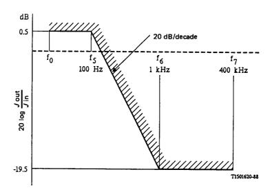
Note I - The frequency  $f_0$  should be less than 20 Hz and as low as possible (e.g. 10 Hz), taking into account the limitations of measuring equipment.
