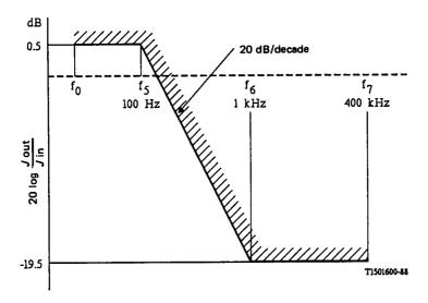
Note 1 - The frequency  $f_0$  should be less than 20 Hz and as low as possible (e.g. 10 Hz), taking into account the limitations of measuring equipment.
