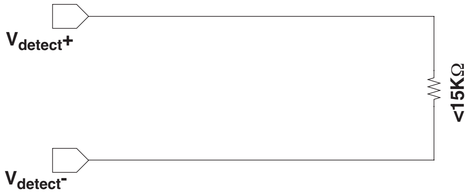
Figure 33A.3—Invalid detection signature, impedance low
