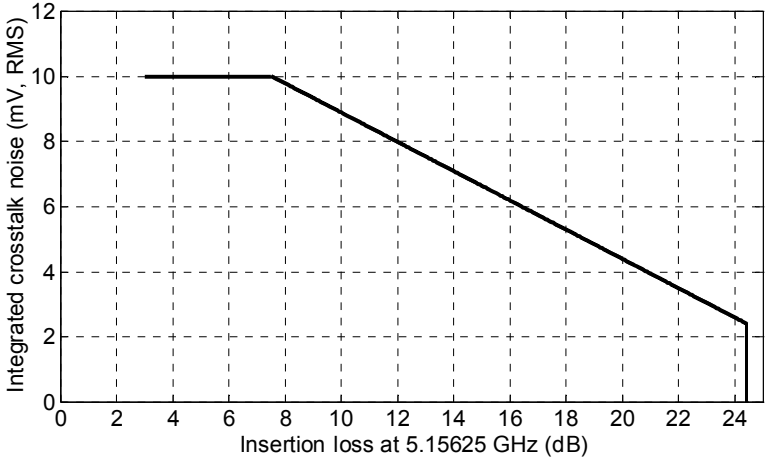
Figure 85A-2—Channel integrated crosstalk noise
