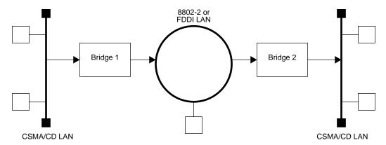
Figure 5—Frame-flow configuration
