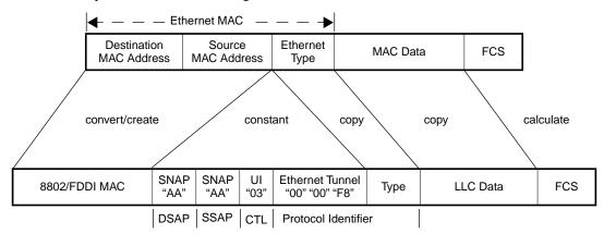
Figure 9—Ethernet Bridge-Tunnel Encapsulation
