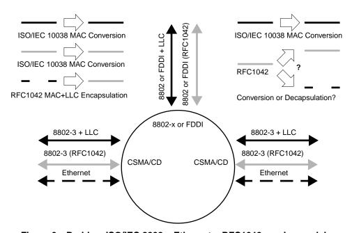
Figure 3—Problem ISO/IEC 8802 + Ethernet + RFC1042 service model
