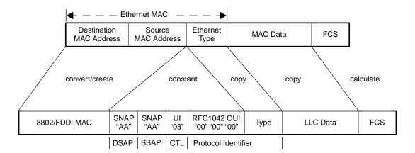
Figure 10—RFC1042 Encapsulation
