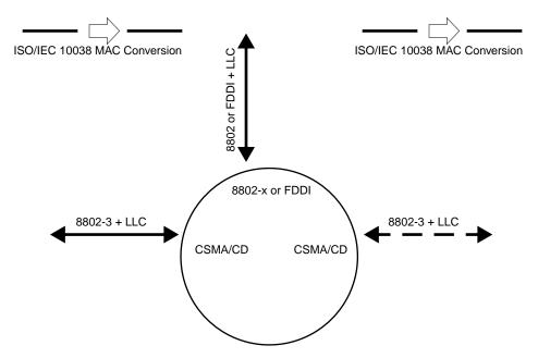
Figure 1—Simple ISO/IEC 8802 service model
