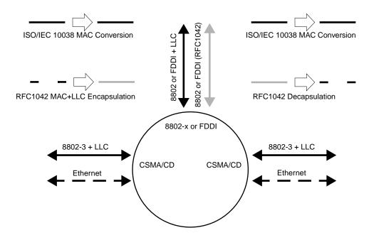
Figure 2—Simple ISO/IEC 8802 + Ethernet service model
