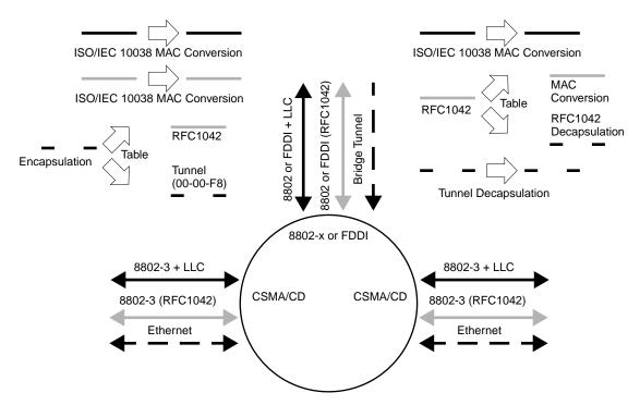
Figure 4—ISO/IEC 8802 + Ethernet + RFC1042 + Bridge-Tunnel service model
