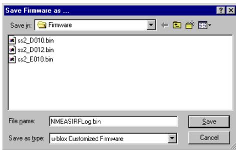
“Save to bin...” allows merging the changes in the user parameters and the original firmware to a new binary file. This customized firmware can be used for an automated download procedure in combination with the command line version, without the need of an additional configuration file.
