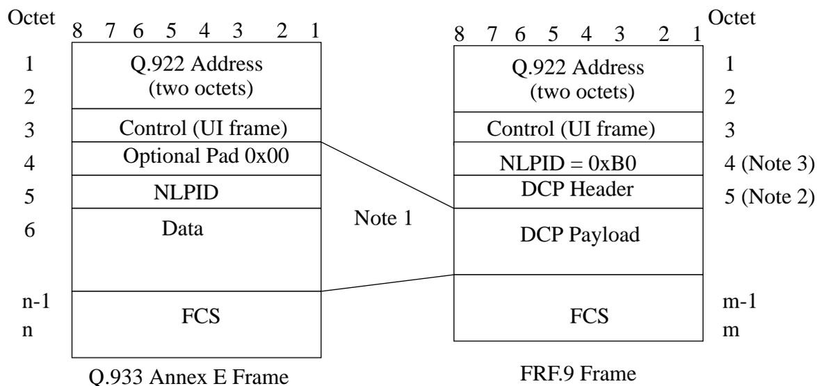
**Figure 1 - Encapsulation of a DCP data PDU that Contains Q.933 Annex E Data**
