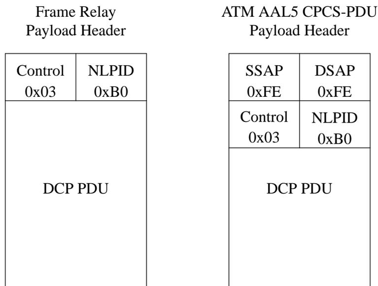
**Figure B.1 - FR/ATM Payload Header Translation for FRF.9 DCP**
