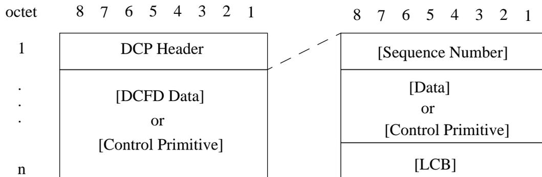
**Figure A.1 - Format of DCP PDU**
