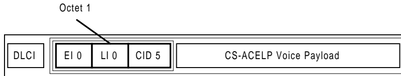
Figure 3-3 Frame containing one sub-frame
