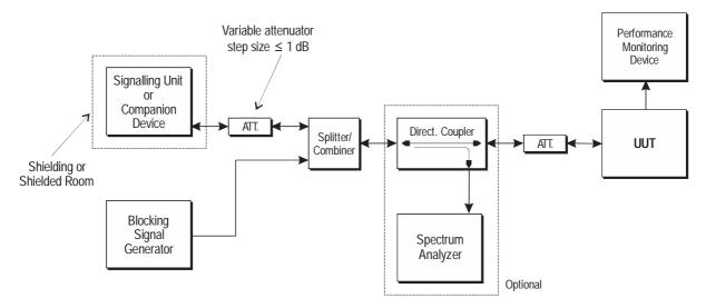
Figure 1: Test Set-up for receiver blocking
