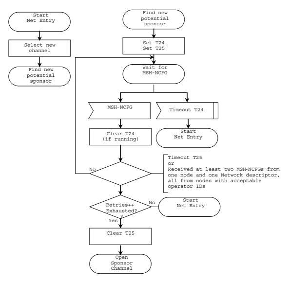
Figure 10: Synchronization and network entry - new node I
