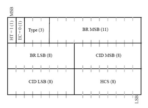
Figure 2: Bandwidth request header format
