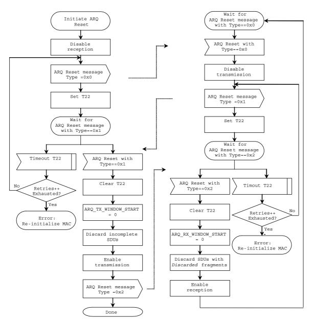
Figure 8: Transmitter initiated ARQ Reset
