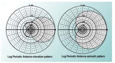
Figure 2: Sample Antenna Directional Pattern
