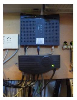
Figure 10: In-home set-up with NIU and cable modem
