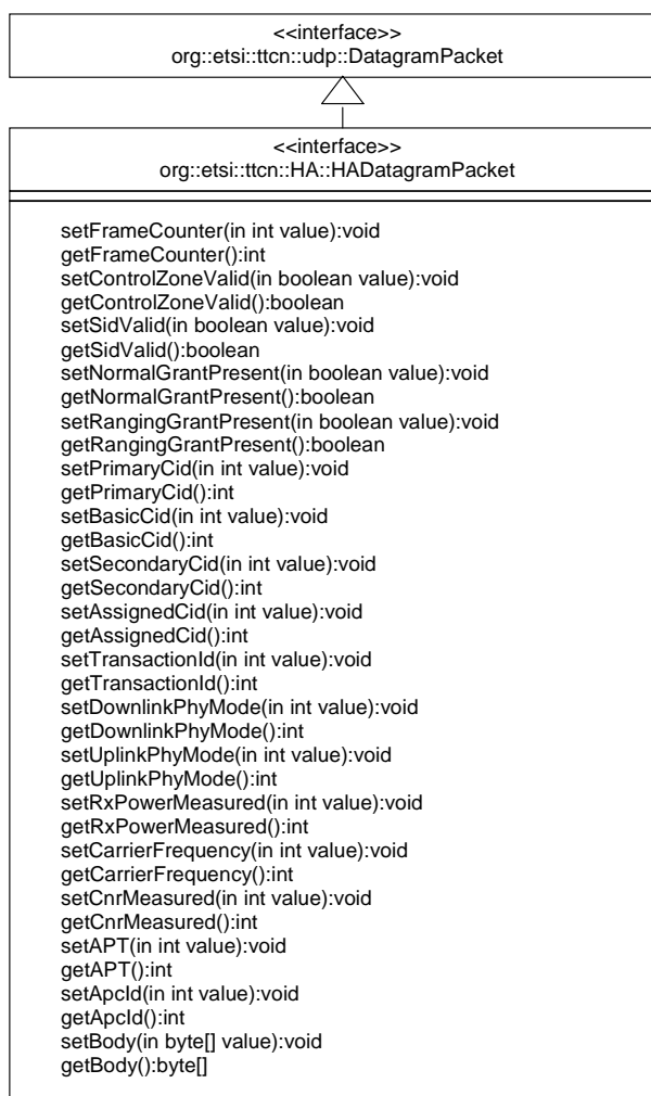
Figure 15: Interface between Test System and UDP datagram
