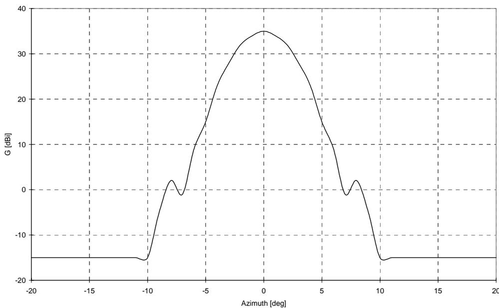
**Figure A.5: Antenna pattern envelope on the azimuth plane**
