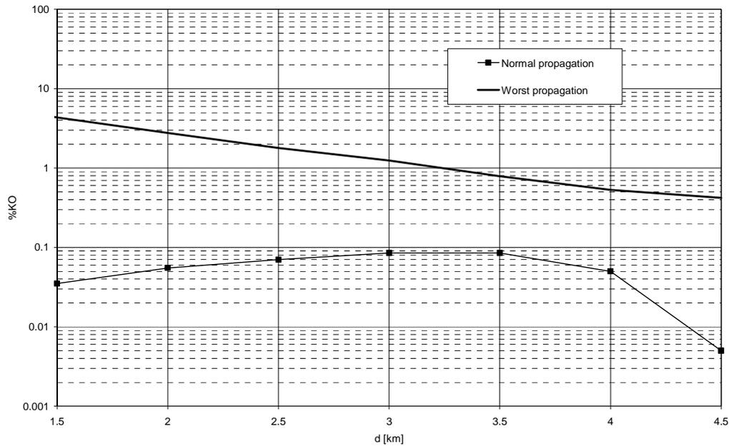
**Figure A.10: %KO area for FDM system (class A1, 28 MHz guard band)**
