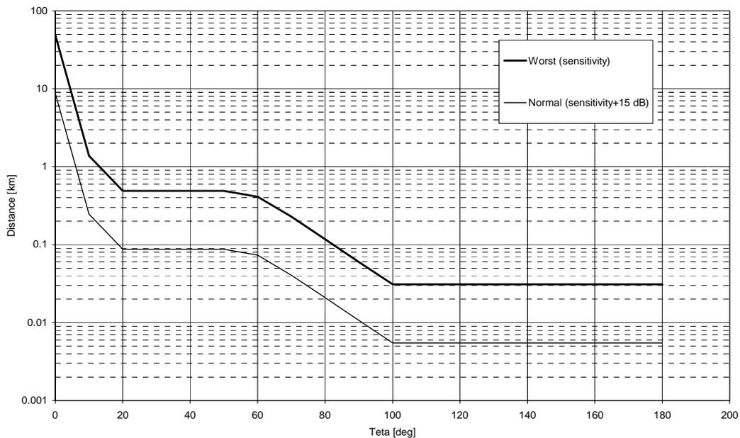
**Figure B.3: Minimum distance between P-P and CRS sites in order to avoid class B1 interference**
