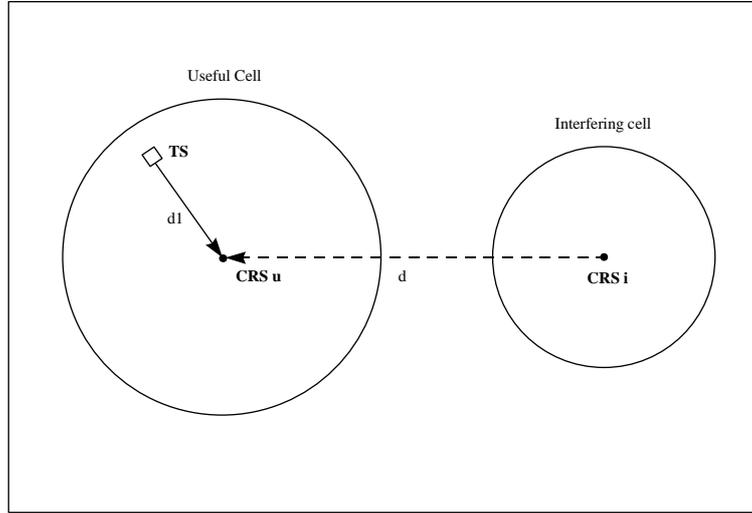
**Figure 7: Generic scenario for class A3 interference analysis**
