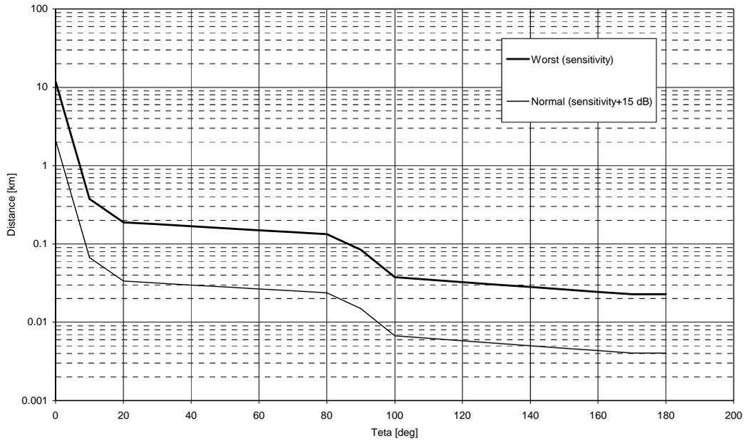
**Figure B.10: Minimum distance between P-P and CRS sites in order to avoid class B1 interference**
