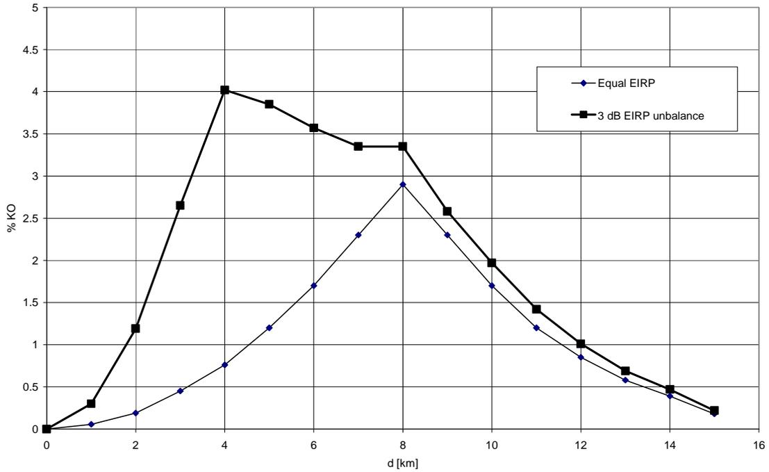
**Figure A.3: %KO area for class A2 (TDM on FHCD) with ETSI limits**
