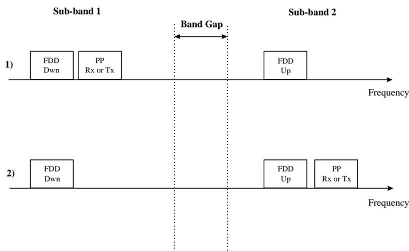
Figure 3: Possible arrangements for a FDD P-MP system and a P-P system
