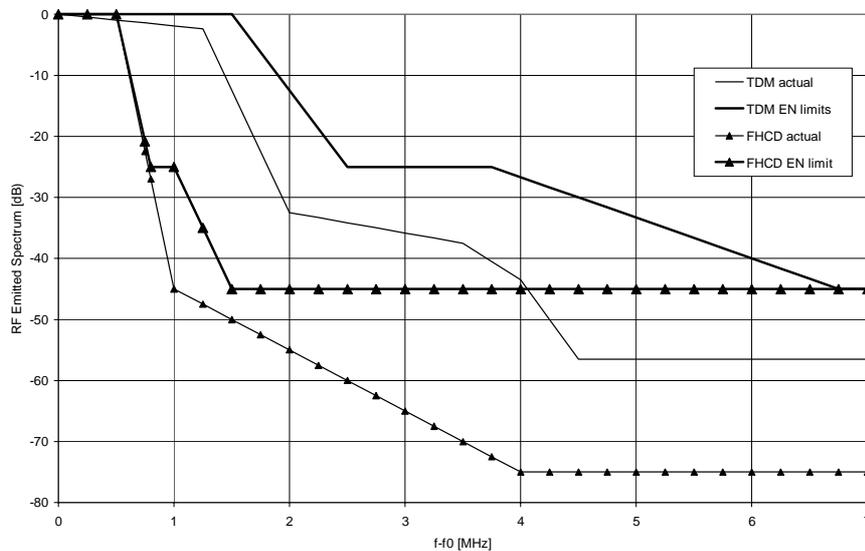
Figure A.1: RF emitted spectrums
