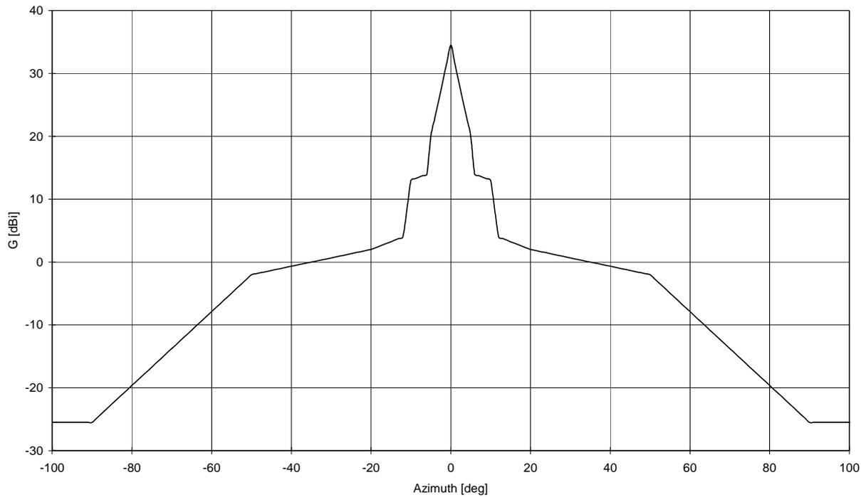
**Figure A.8: TS antenna pattern envelope, on the azimuth plane, for FDM system**
