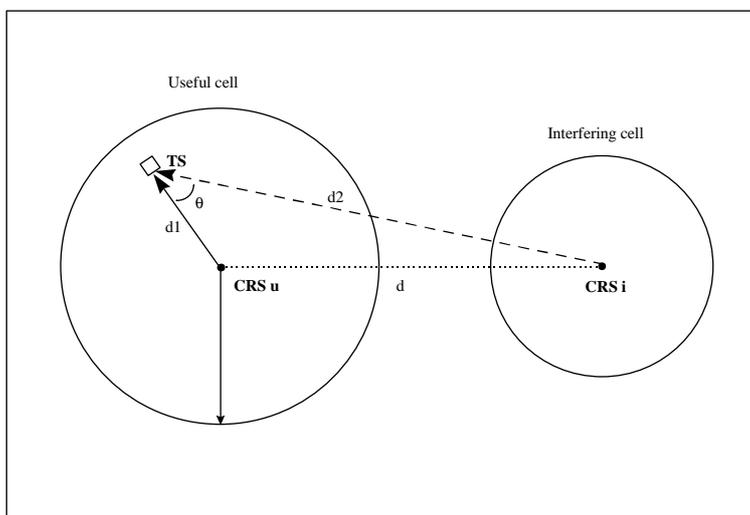
**Figure 5: Generic scenario for class A1 interference analysis**
