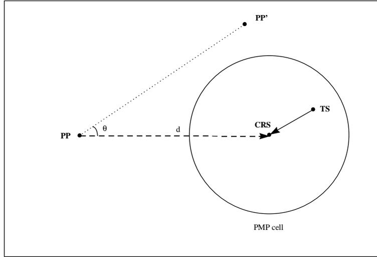
**Figure 11: Generic scenario for class B2 interference analysis**
