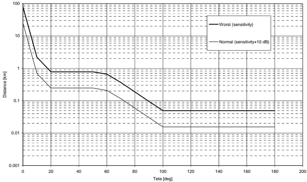
**Figure B.4: Minimum distance between P-P and CRS sites in order to avoid class B2 interference**
