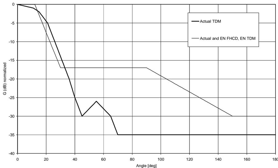
Figure A.2: Antenna pattern envelope on the azimuth plane
