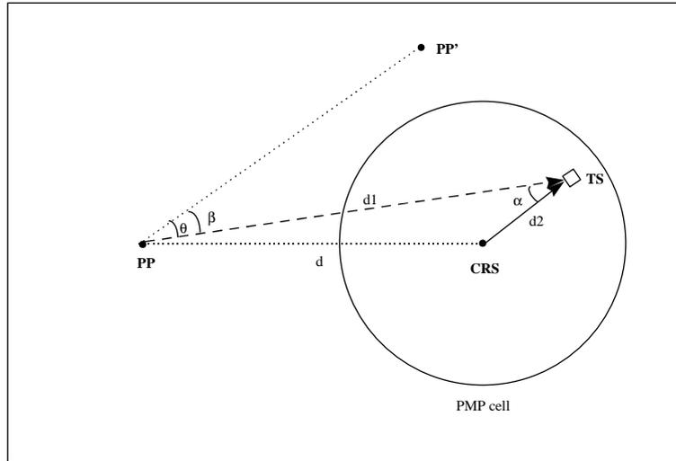
**Figure 13: Generic scenario for class B4 interference analysis**
