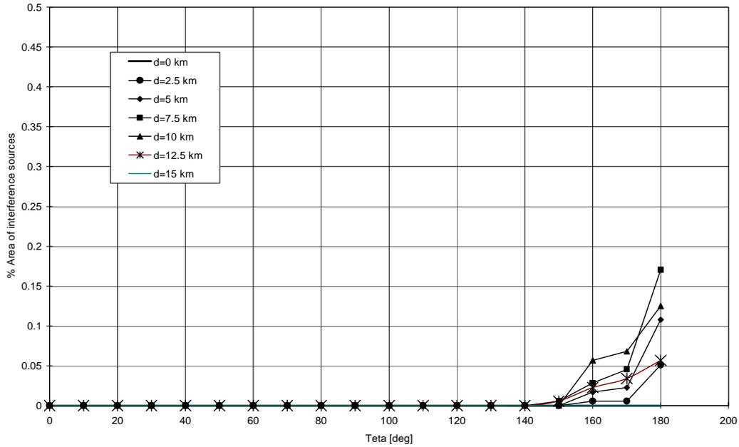
**Figure B.6: % of cell area where any potential TS is interfered by P-P (class B4)**
