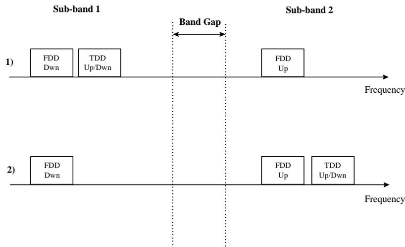
**Figure 2: Possible arrangements for a FDD P-MP system and a TDD P-MP system**
