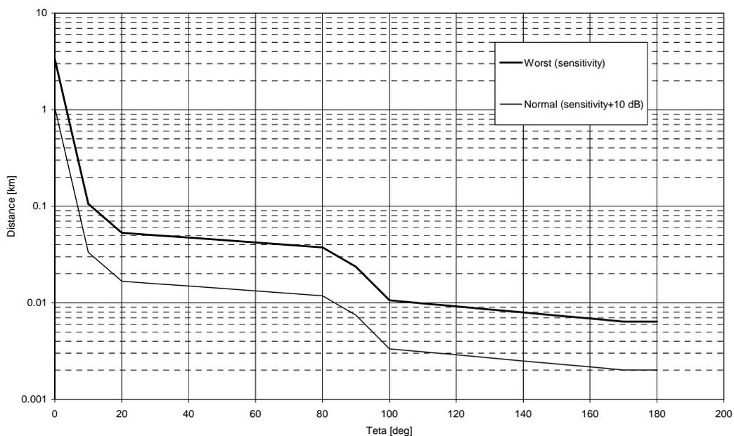
**Figure B.11: Minimum distance between P-P and CRS sites in order to avoid class B2 interference**
