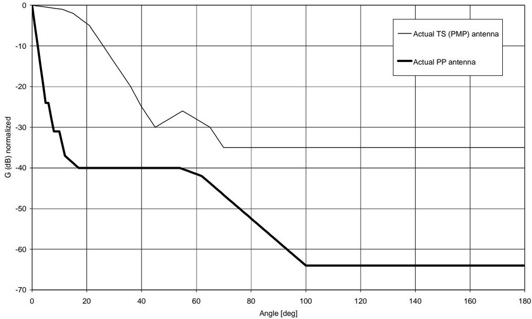
**Figure B.2: Antenna pattern envelope on the azimuth plane**
