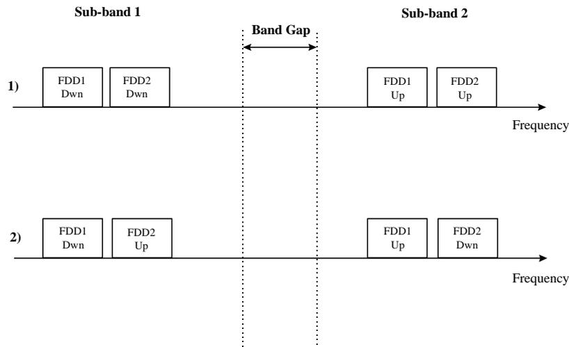
**Figure 1: Possible arrangements for two FDD P-MP systems**
