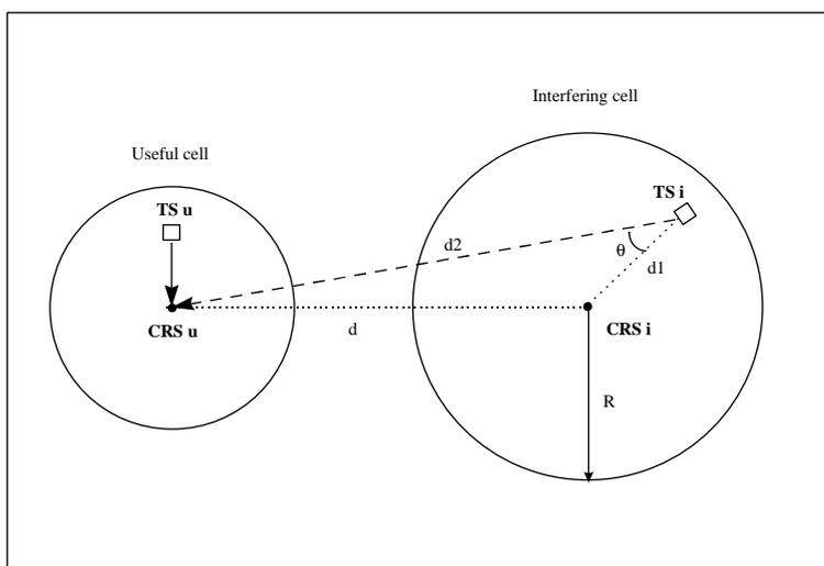
Figure 6: Generic scenario for class A2 interference analysis
