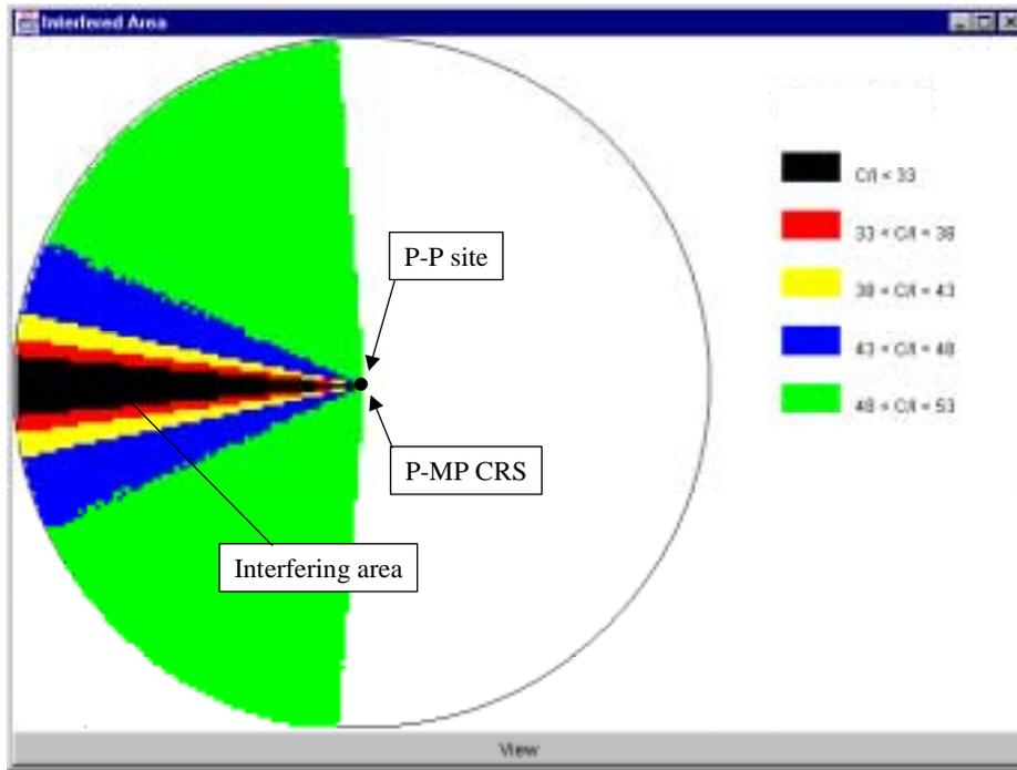
**Figure B.14: Cell area of potential sources (TS) of interference (class B3) and their relevant C/I generated on the P-P receiver**
