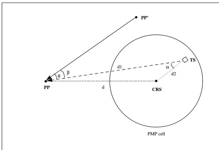
**Figure 12: Generic scenario for class B3 interference analysis**
