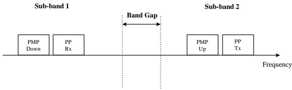
**Figure 14: Useful channel arrangement**
