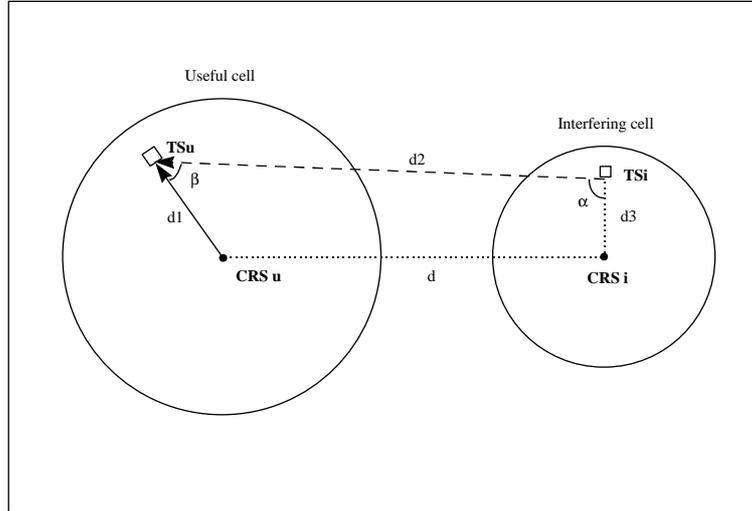
**Figure 8: Generic scenario for class A4 interference analysis**
