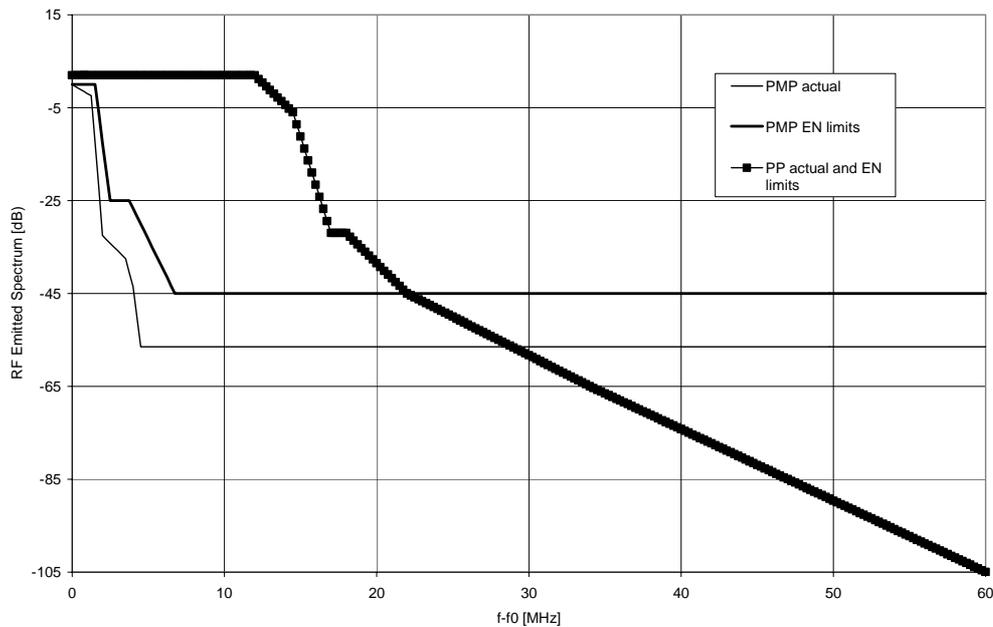
**Figure B.1: RF emitted spectrums**
