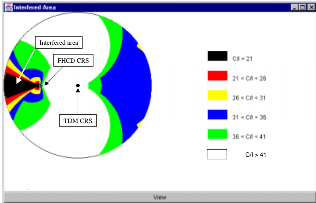
**Figure A.4: C/I distribution over the TDM cell area**
