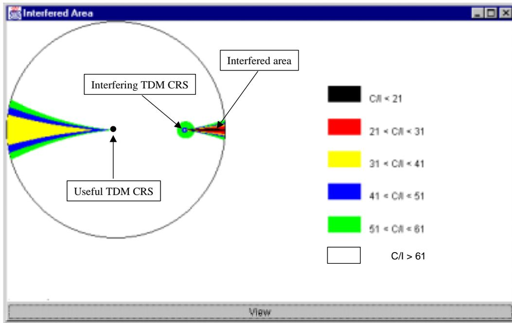
**Figure A.7: C/I distribution over the useful TDM cell area for CRS distance of 2 km**
