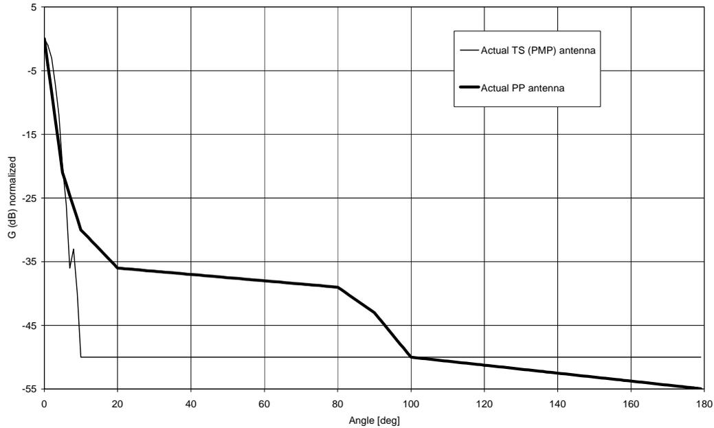
**Figure B.9: Antenna pattern envelope on the azimuth plane**
