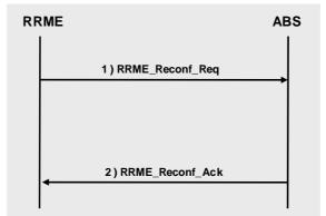
Figure 5.9: Re-configuration request message flow
