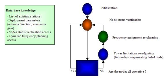
Figure 5.5: Station failure recovery procedure
