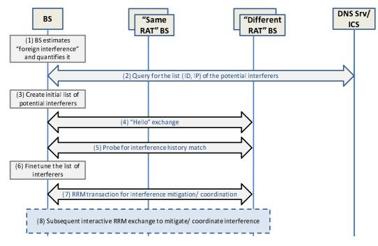
Figure 6.16: Interferer matching, discovery and interference coordination
