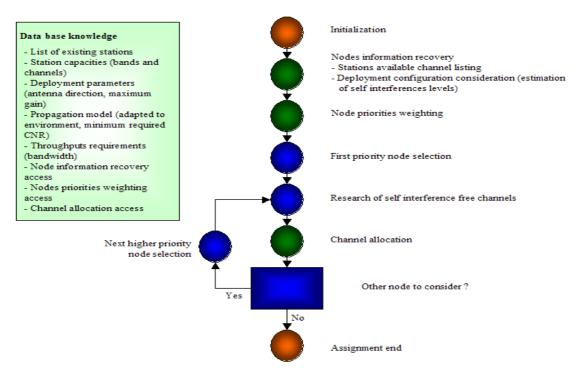
Figure 5.1: Dynamic frequency planning algorithm
