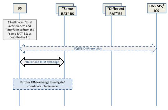
Figure 6.15: Interference detection
