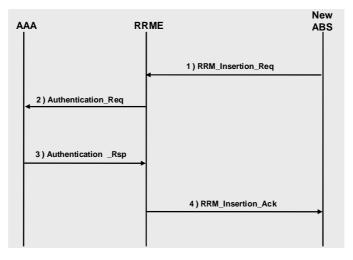
Figure 5.7: A new station insertion message flow
