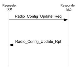
Figure 6.7: Radio Configuration update (Pull)
