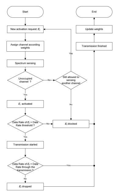
Figure 5.13: Reinforcement learning based channel assignment algorithm
