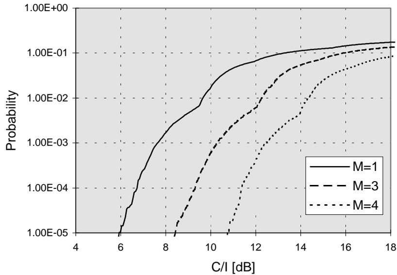
Figure 12: C/I cumulative distribution function for TDMA, FDMA and FH-CDMA with antenna in figure 6 and interfering propagation exponent  $\gamma = 2$
