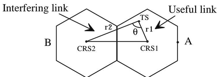
**Figure 3: Example of interference in a TS-CRS connection**
