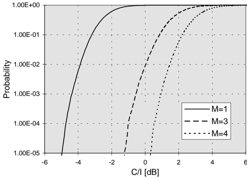
Figure 7: C/I cumulative distribution function for Pseudo Random DS-CDMA with antenna in figure 5 and interfering propagation exponent  $\gamma = 2$
