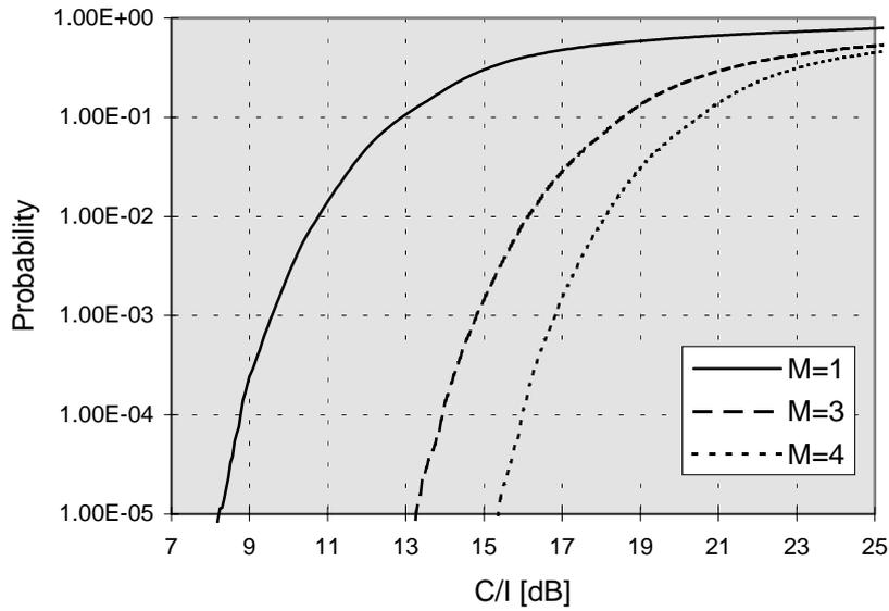
Figure 13: C/I cumulative distribution function for TDMA, FDMA and FH-CDMA with antenna in figure 5 and interfering propagation exponent  $\gamma = 3$
