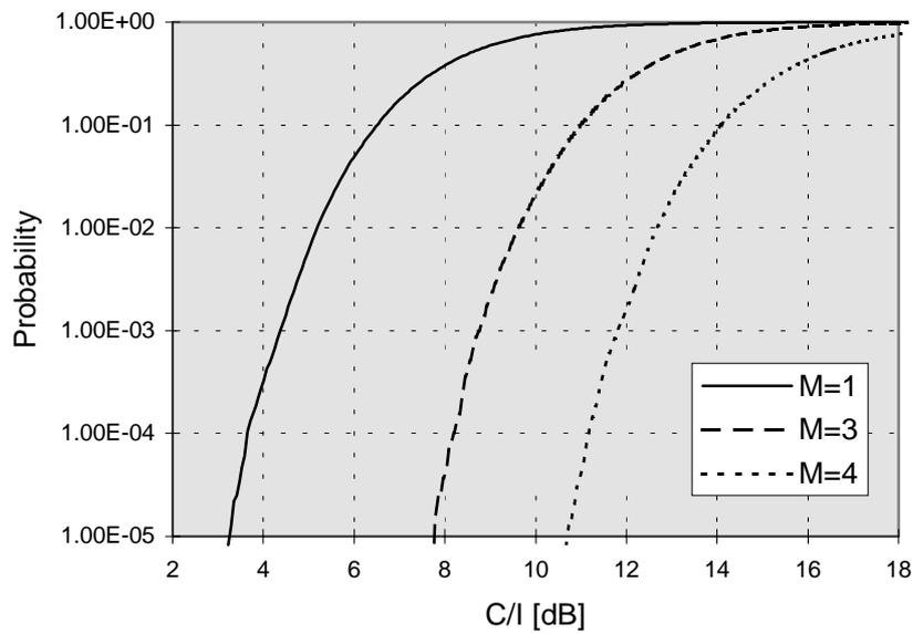
Figure 10: C/I cumulative distribution function for Pseudo Random DS-CDMA with antenna in figure 6 and interfering propagation exponent  $\gamma = 3$
