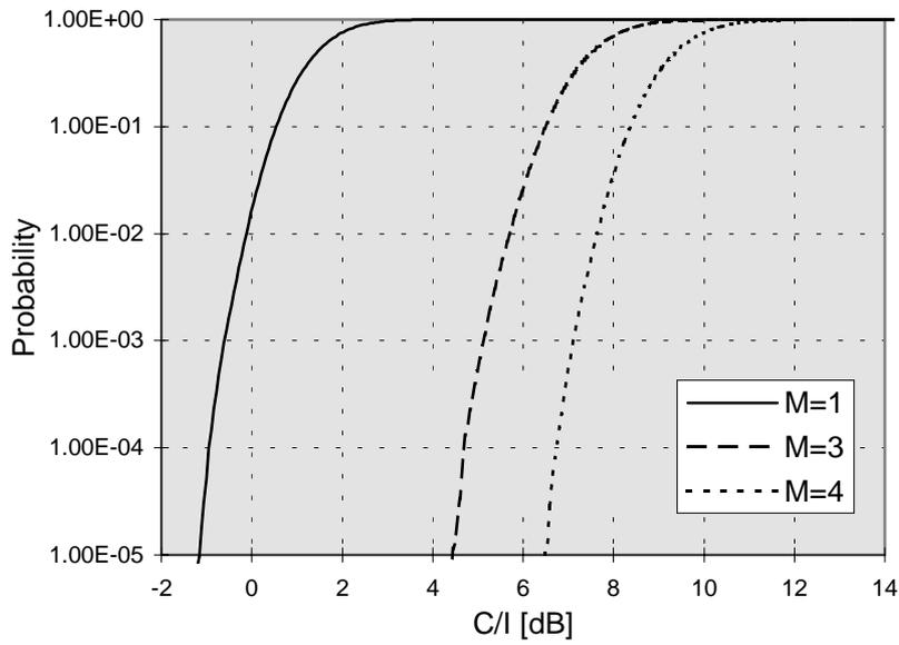
Figure 9: C/I cumulative distribution function for Pseudo Random DS-CDMA with antenna in figure 5 and interfering propagation exponent  $\gamma = 3$
