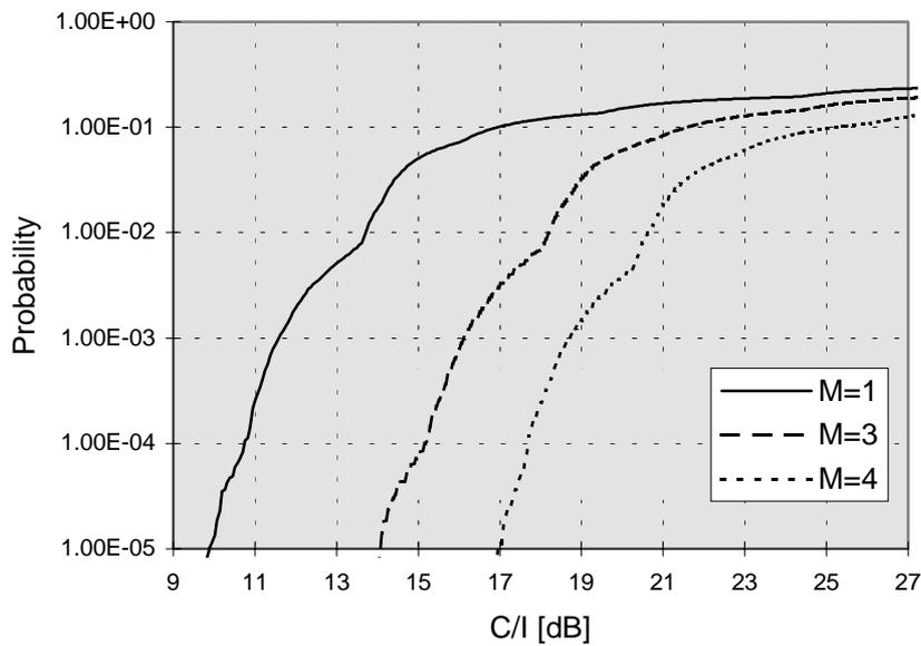
Figure 14: C/I cumulative distribution function for TDMA, FDMA and FH-CDMA with antenna in figure 6 and interfering propagation exponent  $\gamma = 3$
