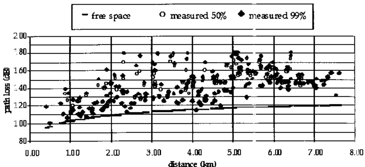
Figure A.1: path loss measurements
