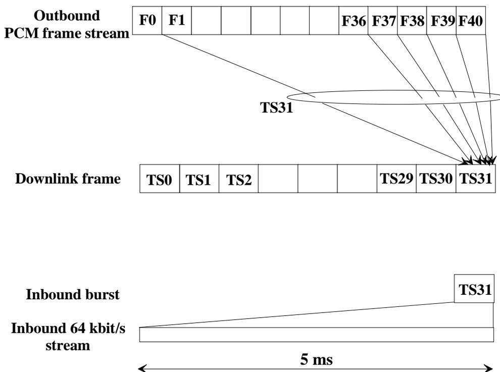
Figure 4: TDMA frame format
