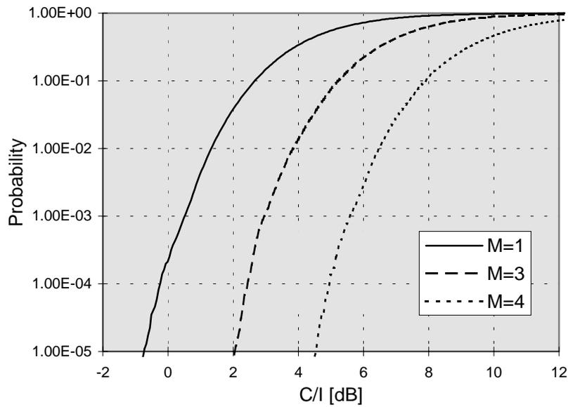
Figure 8: C/I cumulative distribution function for Pseudo Random DS-CDMA with antenna in figure 6 and interfering propagation exponent  $\gamma = 2$
