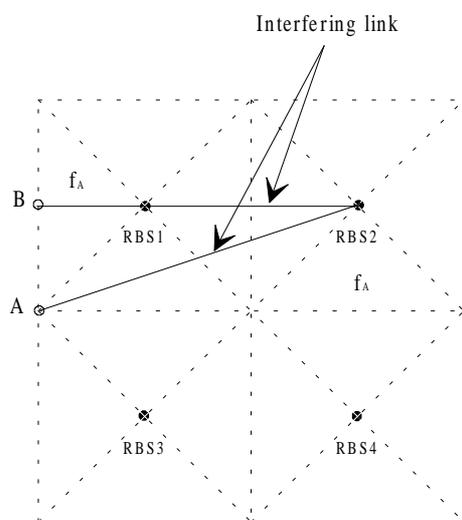
**Figure 4: Example of interference in a TS-CRS connection with 90° sectored antenna**
