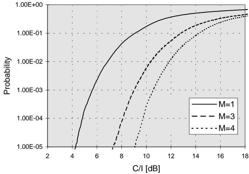
Figure 11: C/I cumulative distribution function for TDMA, FDMA and FH-CDMA with antenna in figure 5 and interfering propagation exponent  $\gamma = 2$
