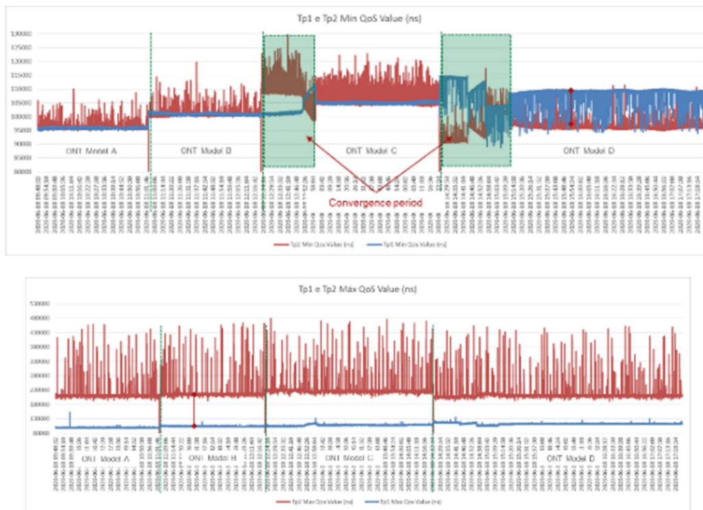
Figure 8: Example of PDV for downlink (Tp1) and uplink (Tp2) measured in a GPON solution
