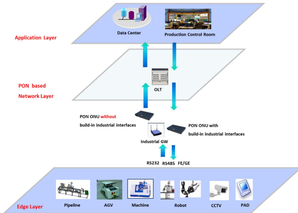
Figure 3: The architecture of the industrial interfaces and protocols carried by a PON system
