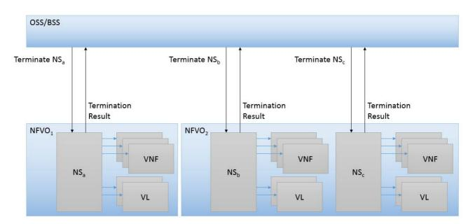
Figure 5.17.1.2-1: Terminate NS requests sent to each NFVO for the NSs that are part of the end-to-end service
