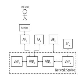
Figure 5.24.1-1: A Service instance consists of Afs as an overlay on VNFs
