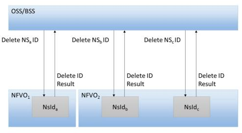
Figure 5.17.1.2-2: Delete nsld requests sent to each NFVO for the NSs that are part of the end-to-end service
