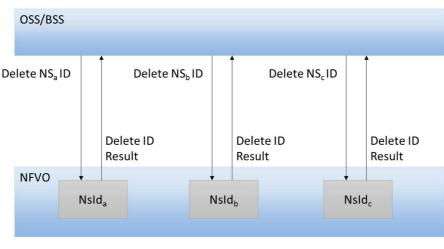
Figure 5.17.1-2: Delete nsId requests sent to the NFVO for the NSs that are part of the end-to-end service
