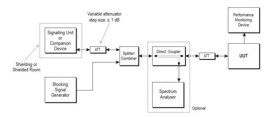
Figure 12: Test set up for receiver blocking
