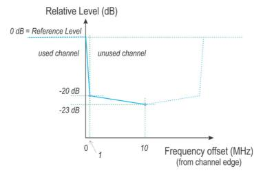
Figure 4: Channel edge mask - case 3
