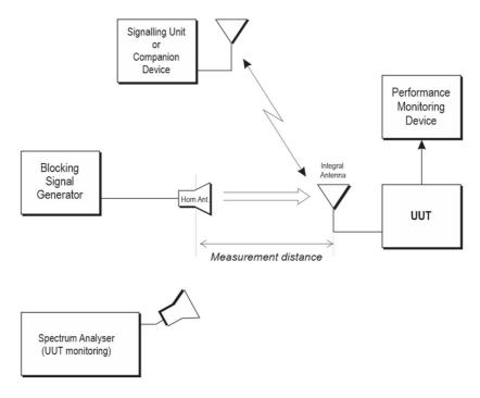
Figure C.4: Measurement set up
