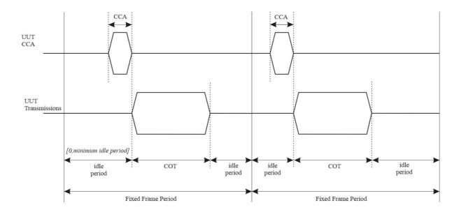
Figure 5: Example of timing for FBE
