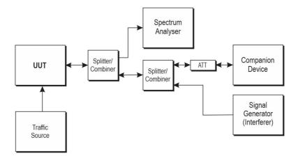
Figure 10: Example test set up for verifying the channel access mechanism of LBE
