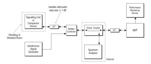
Figure 13: Test set up for receiver selectivity
