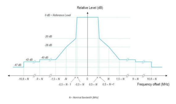
Figure 1: Transmit spectral power mask
