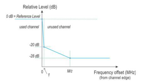
Figure 2: Channel edge mask - case 1
