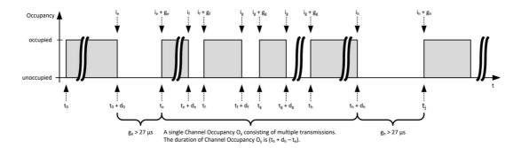
Figure 11: Example of UUT transmissions
