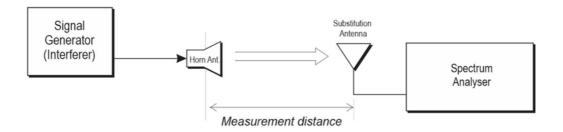
Figure C.3: Measurement set up for calibration
