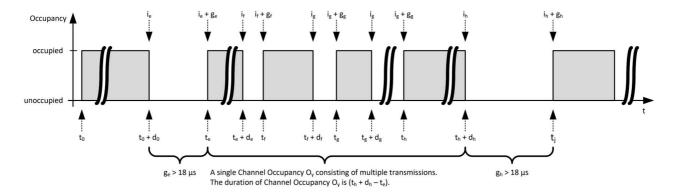
Figure 9: Example of UUT transmissions
