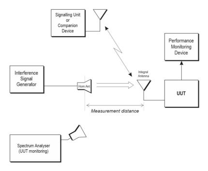
Figure C.6: Measurement set up
