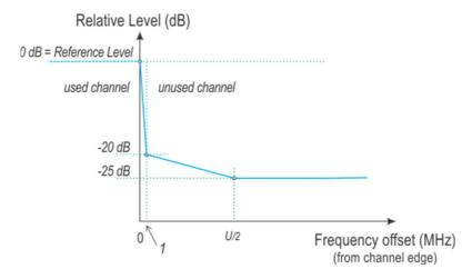
Figure 3: Channel edge mask - case 2
