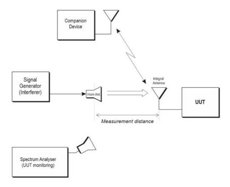
Figure C.2: Measurement set up
