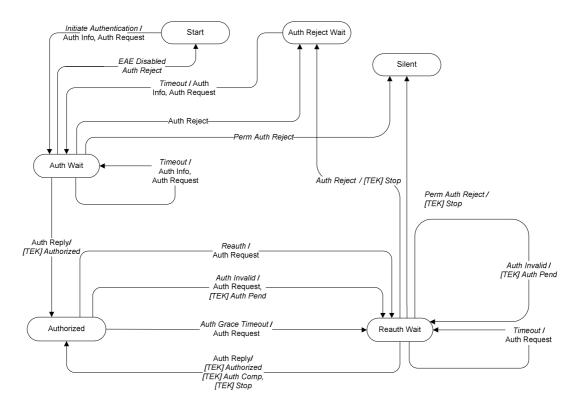
Figure 7-2: Authorization State Machine Flow Diagram
