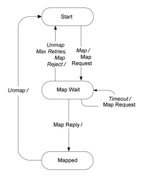
Figure C-1: SA Mapping State Machine Flow Diagram
