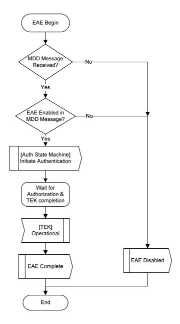
Figure 8-1: EAE Signaling Flow Chart for CM
