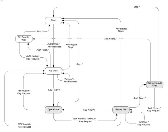
Figure 7-3: TEK State Machine Flow Diagram
