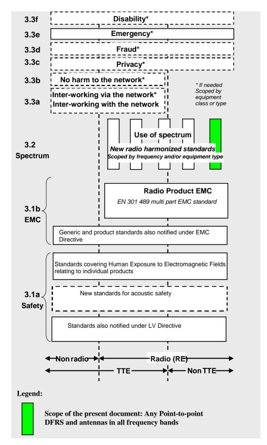
Figure 1: Modular structure for the various standards used under the R&TTE Directive [2]
