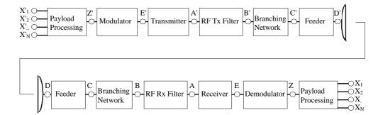
Figure 3: RF system block diagram
