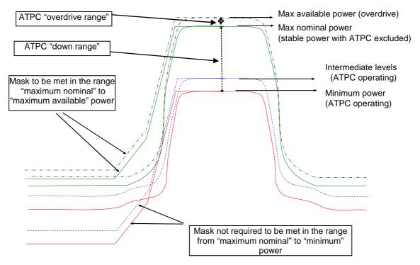
Figure D.1: Relationship between spectrum mask requirement and ATPC operation
