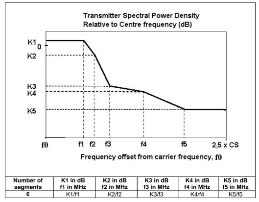
Figure 5: Six segment spectrum mask
