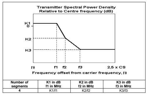
Figure 3: Four segment spectrum mask
