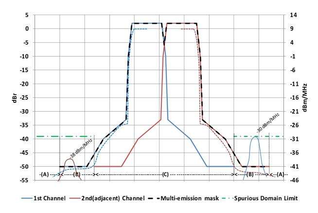
Figure O.7: Example of combined limits in adjacent channels conditions (23 GHz to 28 GHz band; class 4H; Pout = +23 dBm; symbol frequency 25 MHz)
