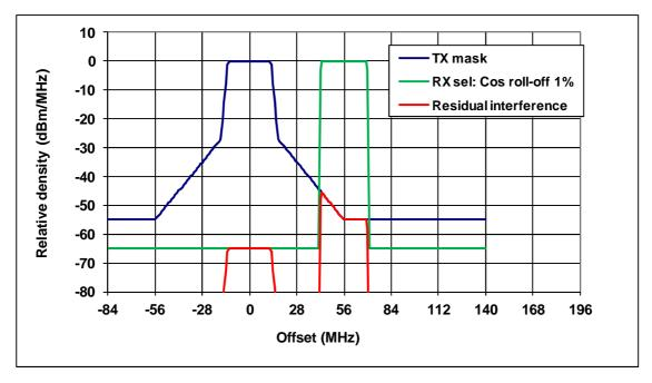
Figure P.2: Example of NFD<sub>2A</sub> evaluation (CS 28 MHz, class 4, roll-off 1 % resulting in NFD<sub>2A</sub> = 50,91 dB)
