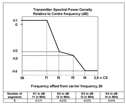
Figure 4: Five segment spectrum mask
