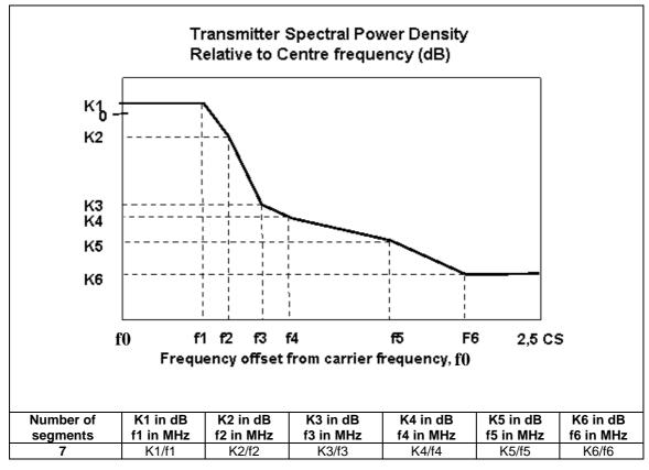
Figure 6: Seven segment spectrum mask
