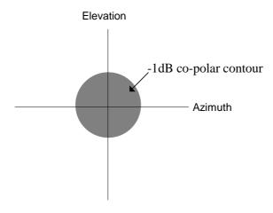
Figure 3: Mask for the antenna XPD measurements around the main beam axis (figure 8)
