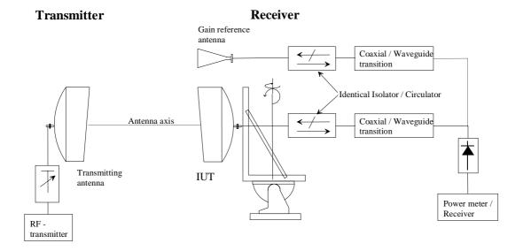
Figure 7a: Test set-up for gain measurement with substitution method using coaxial cables
