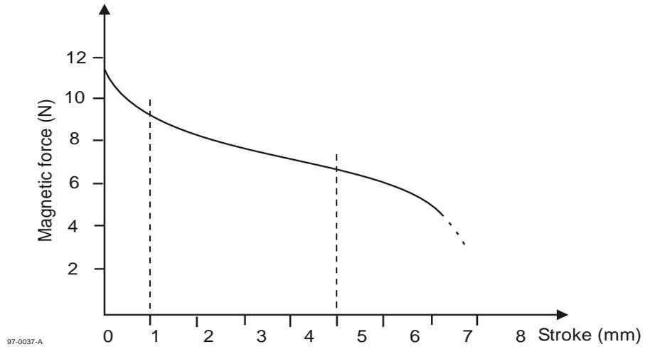
**Figure A.2 — Solenoid characteristics for a plunger stroke of 4 mm**
