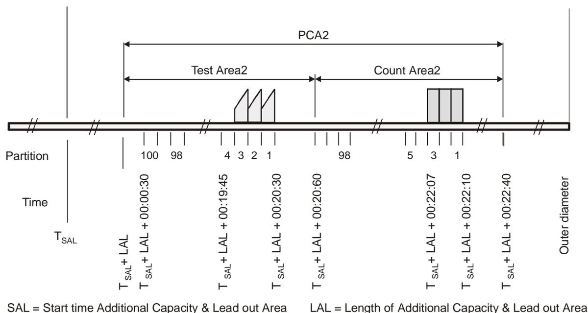
**Figure 12-9 Organization of the PCA2 area in the Additional Capacity & Lead out Area**
