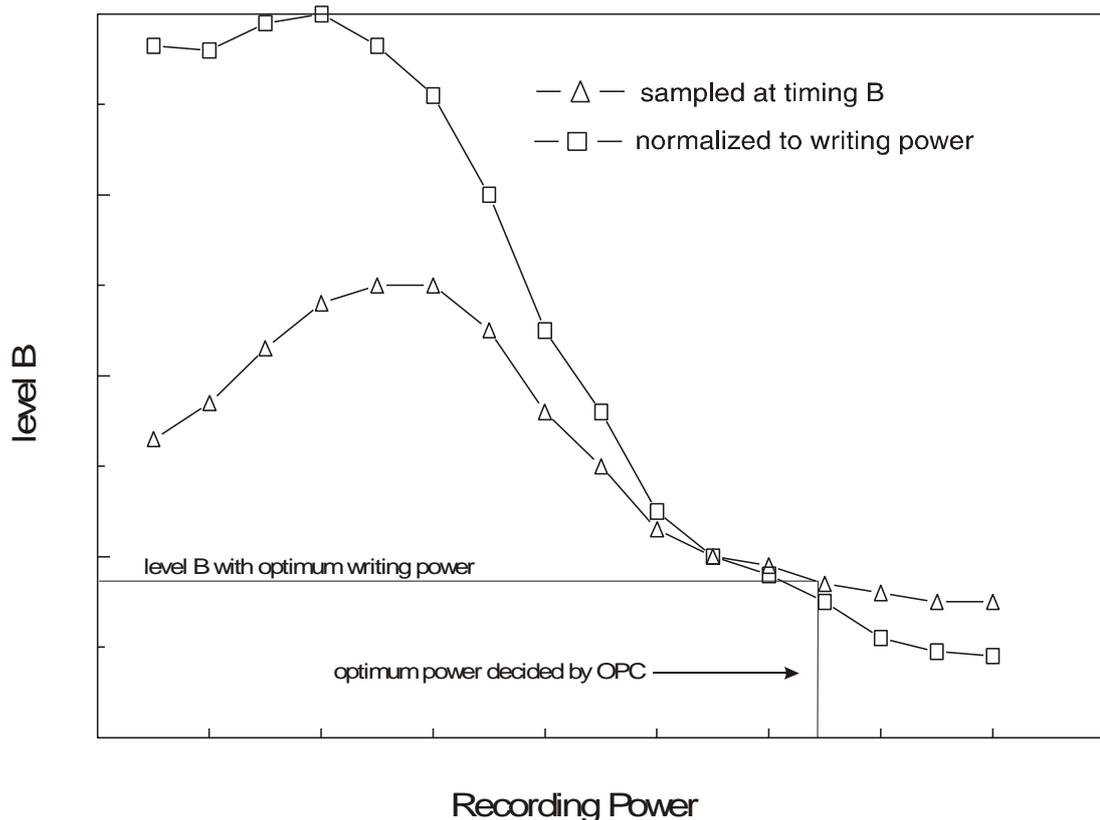
**Figure 13-15 Example of reflected B-level as a function of writing power (11T pulses)**
