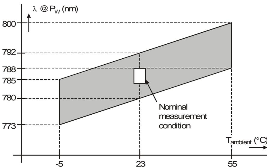
Figure 13-8 Wavelength/Temperature diagram indicating the disc operating conditions
