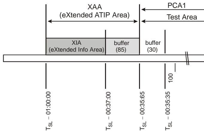
Figure 12-7 Details of Extended ATIP Area (XAA)
