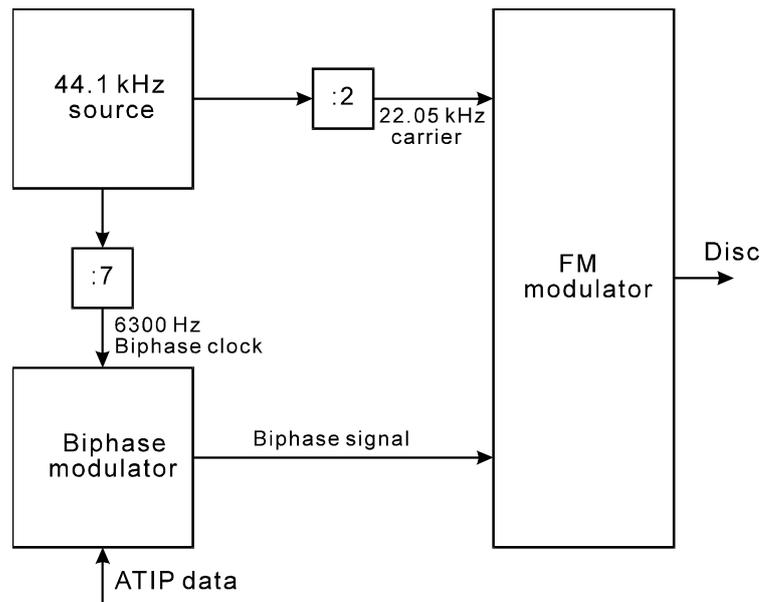
**Figure 4-14 Block diagram of a typical ATIP encoder**
