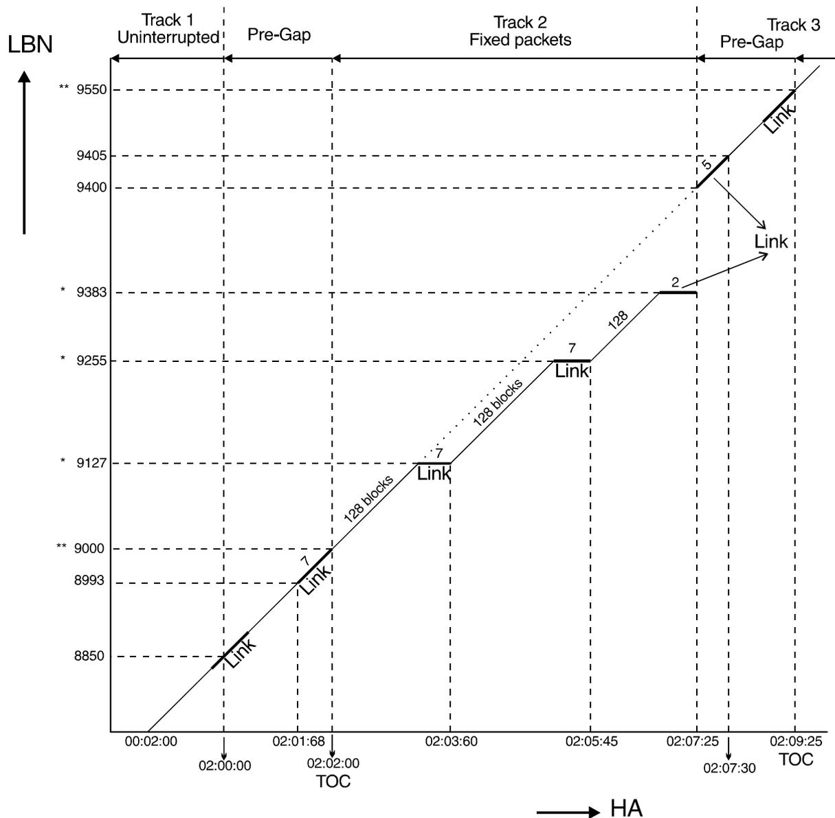
Figure 13-10 Example of addressing Method 1 and 2
