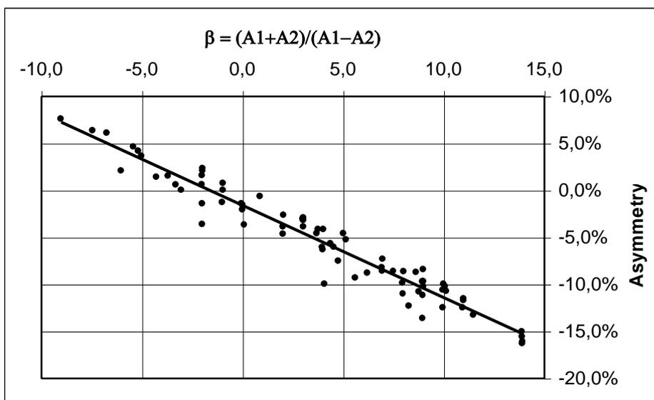
Figure 13-5 Relation between  $\beta$  and asymmetry (experimentally determined)
