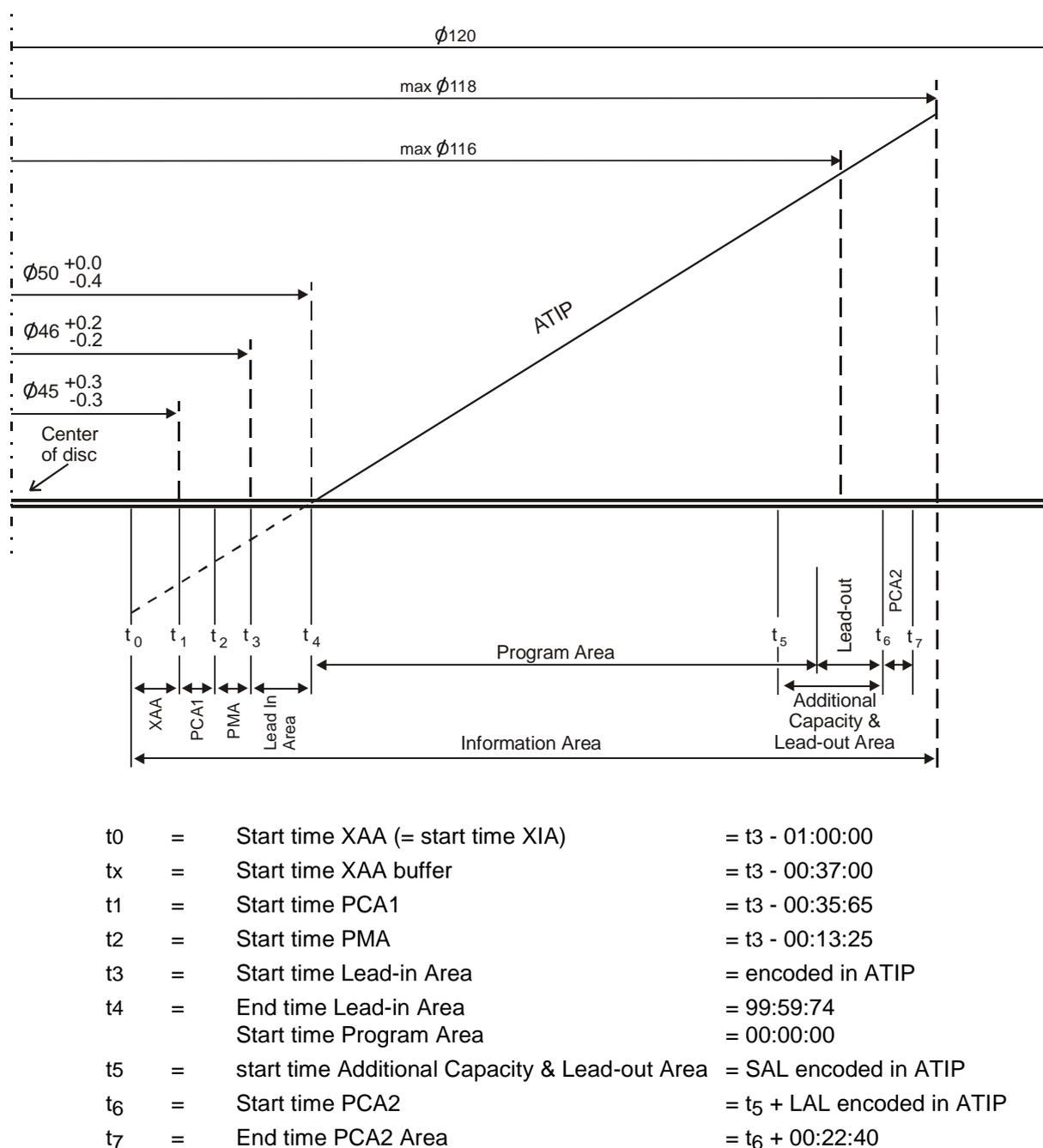
**Figure 12-6 ATIP versus disc diameters**
