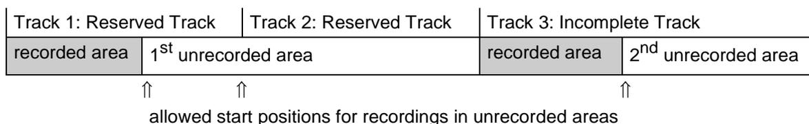
**Figure 5-7 Example of start positions for recordings in unrecorded areas**
