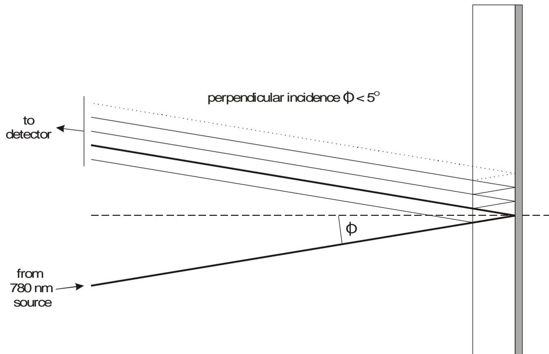
Figure 13-2 Schematic set-up for calibration of reference disc
