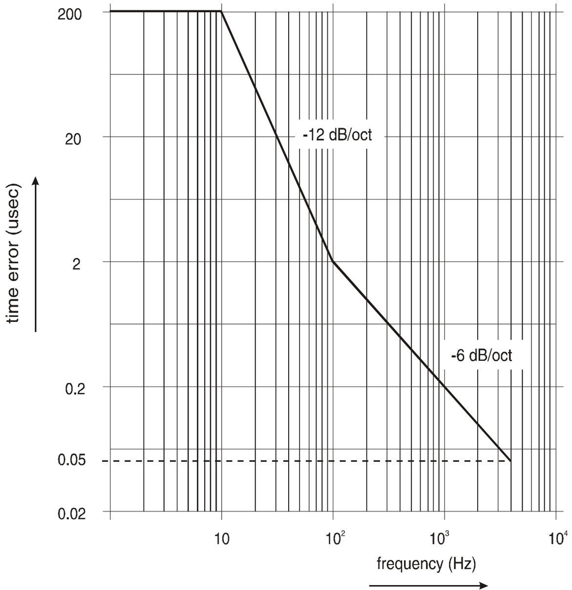
Figure 12-5 Maximum allowed time errors versus frequency spectrum
