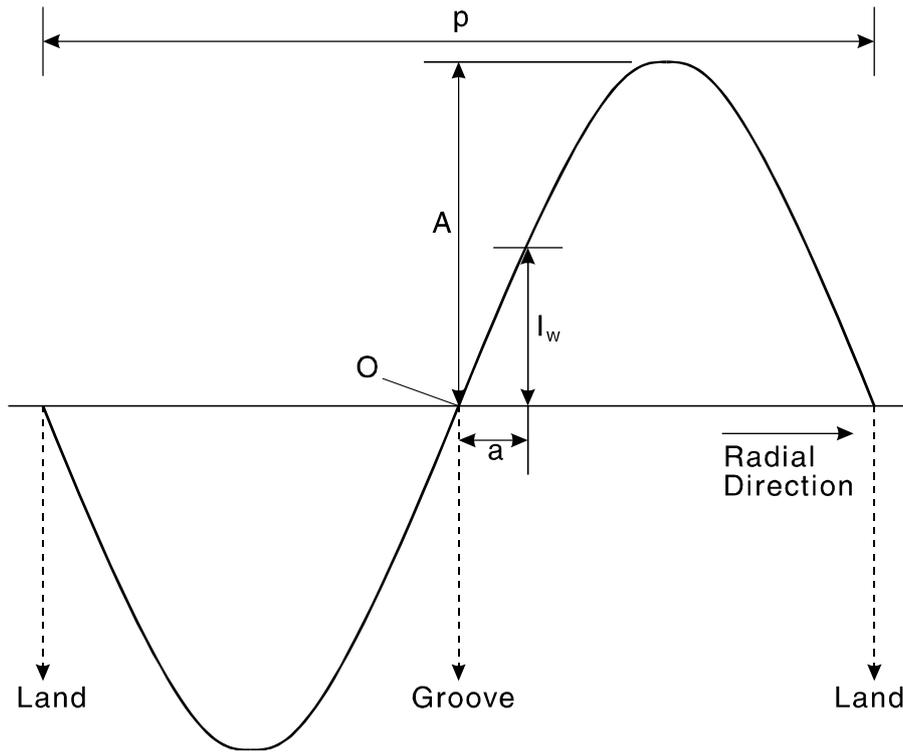
Figure 13-6 The radial error signal
