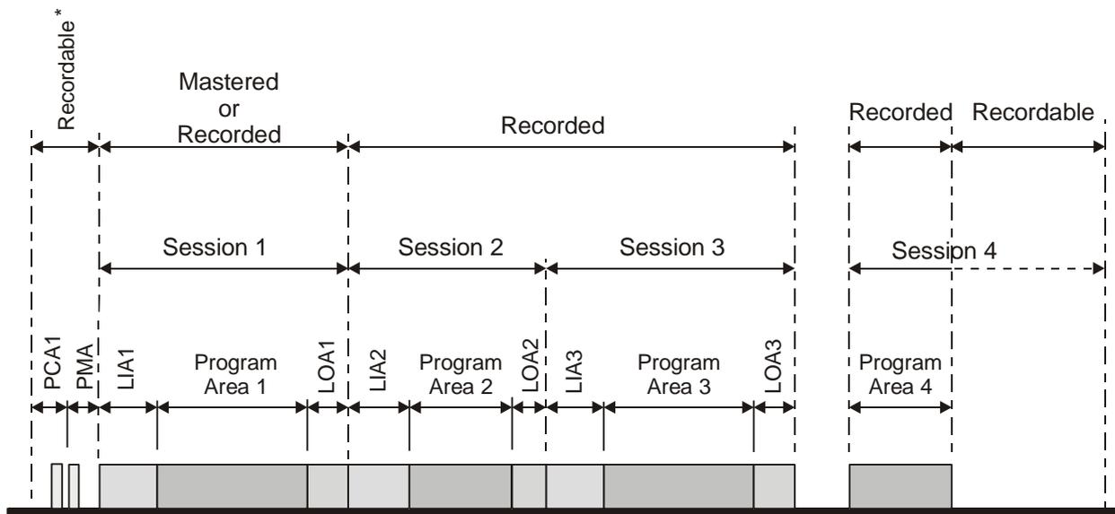
**Figure 12-18** Example of the layout of a Multisession disc
