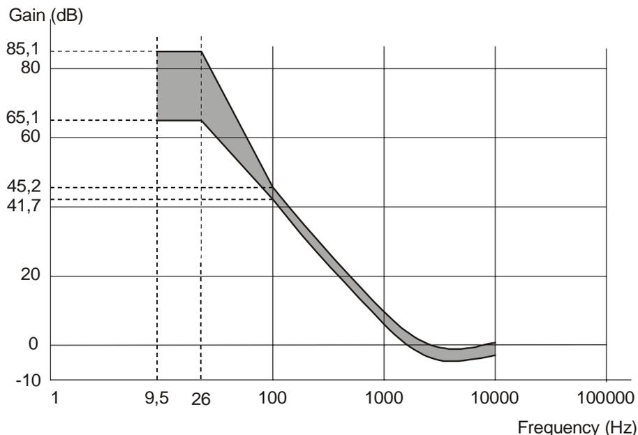
Figure 4 - Reference servo for axial tracking
