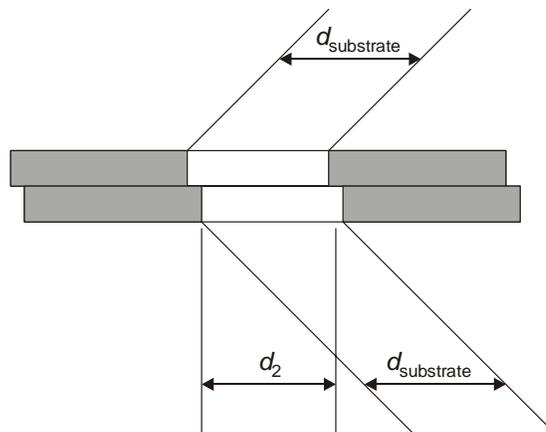
*Figure 7 - Hole diameters for an assembled disk*
