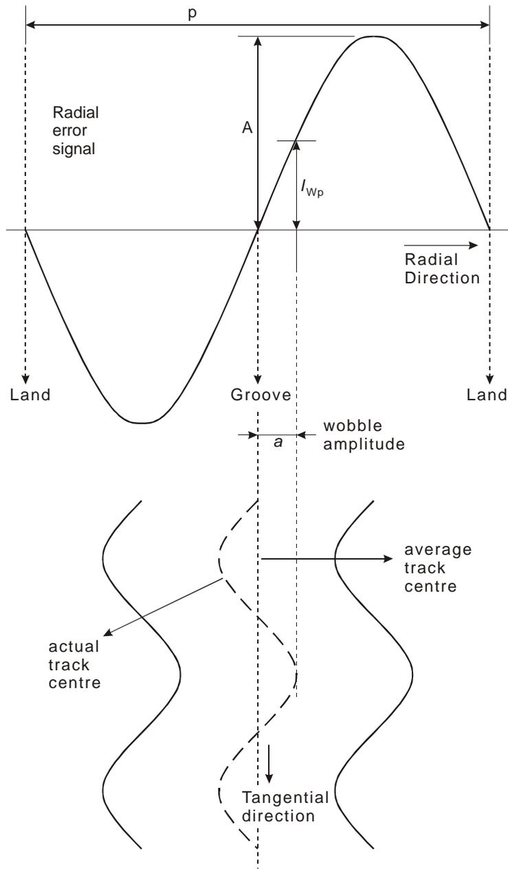
Figure L.1 - Wobble amplitude of the groove
