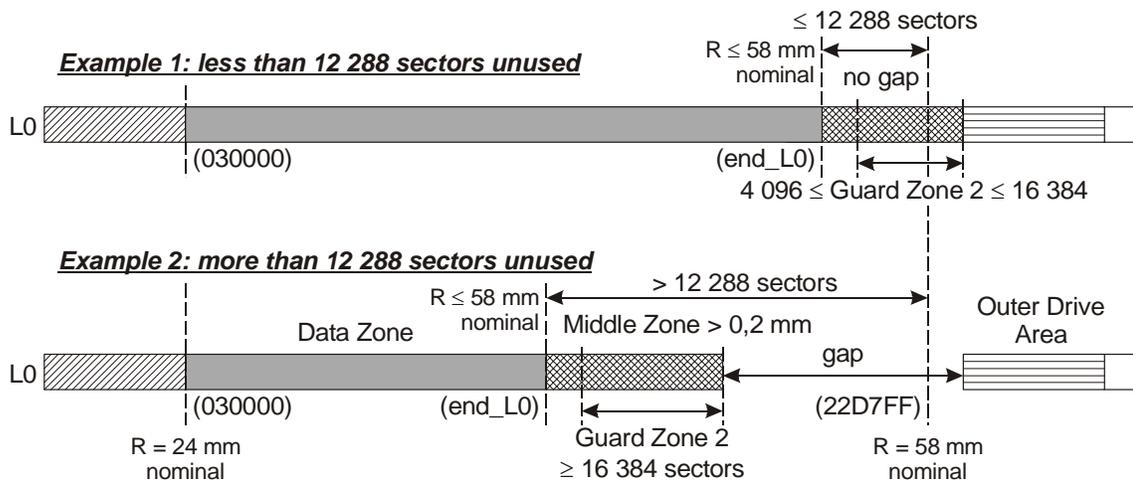
Figure 30 - Two examples of size of Guard Zone 2 on Layer 0
