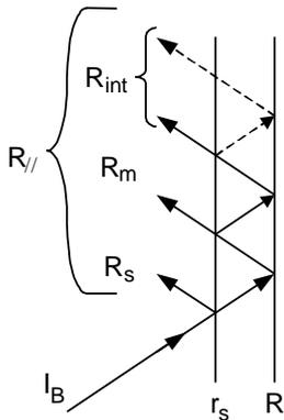
*Figure C.1 - Reflectivity calibration*
