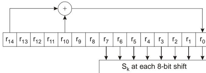
Figure 13 - Feedback shift register
