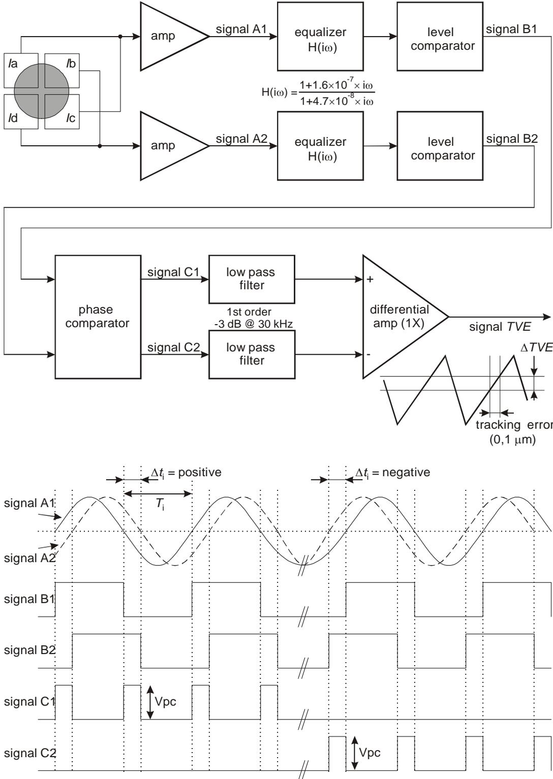
Figure F.1 - Circuit for tracking error measurements
