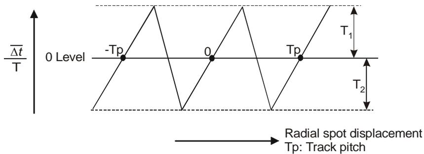
Figure 41 - Differential phase tracking error signal
