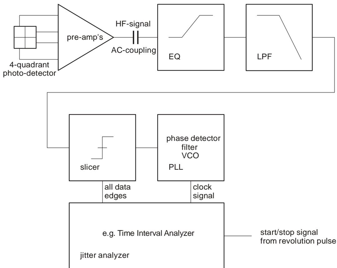
*Figure E.1 - General diagram for jitter measurement*
