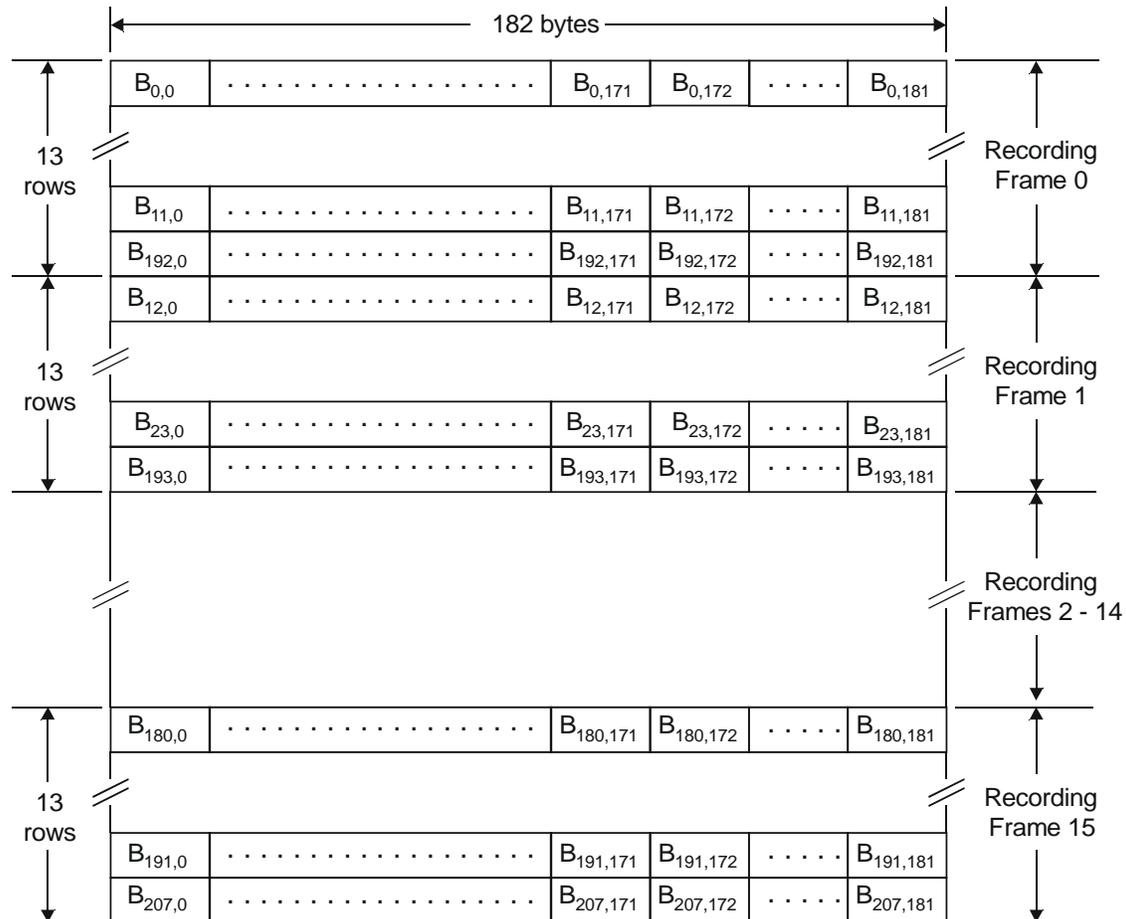
Figure 15 - Recording Frames obtained from an ECC Block
