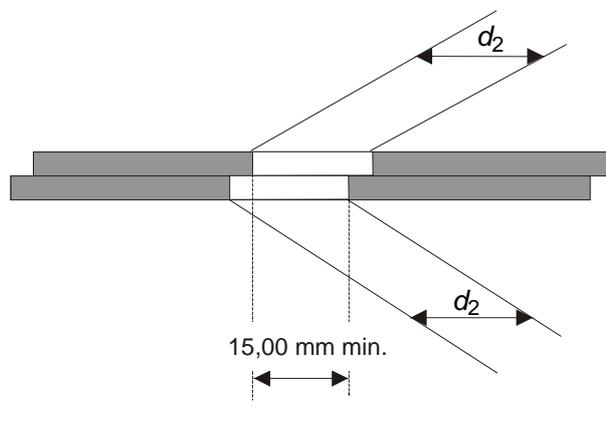
Figure 8 - Hole of the assembled disk
