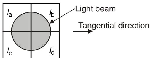
Figure 12 - Quadrant photo detector
