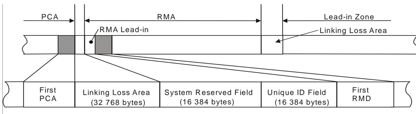
Figure 59 - Layout of the Recording Management Area
