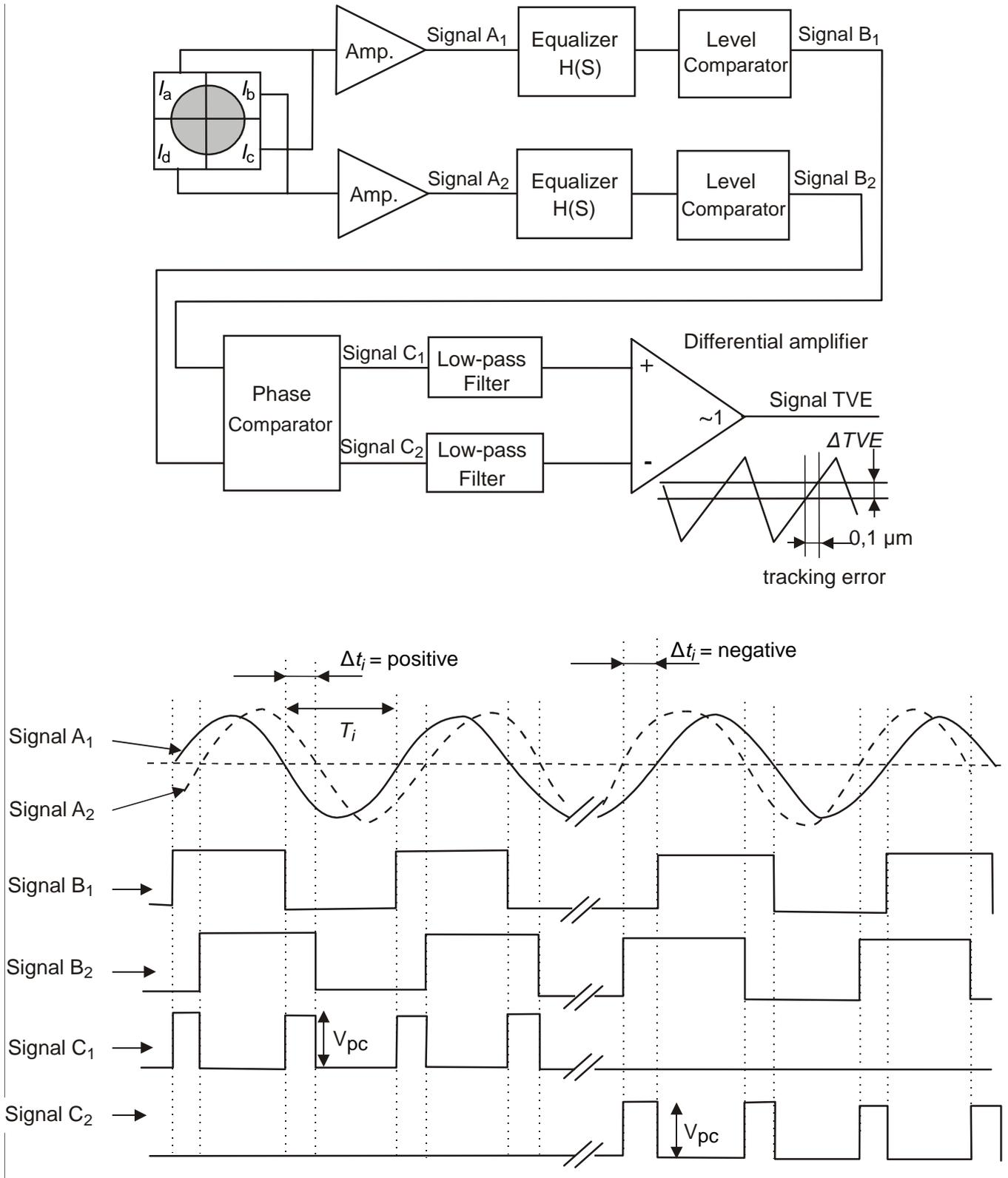
Figure C.1 - Circuit for tracking error measurements
