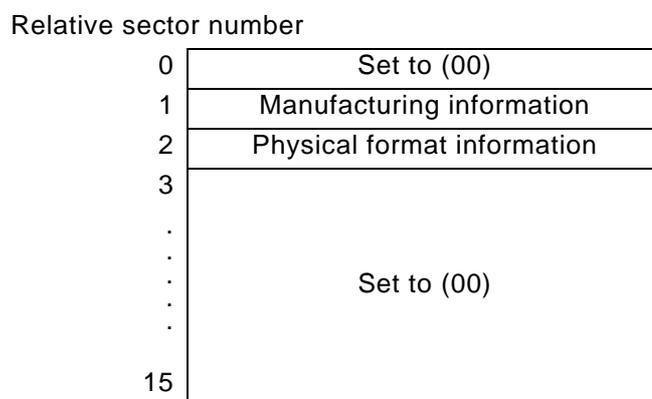
*Figure 37 – Structure of a R-Physical format information block*
