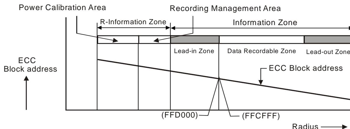
Figure 40 - Pre-pit sector layout and ECC Block numbering
