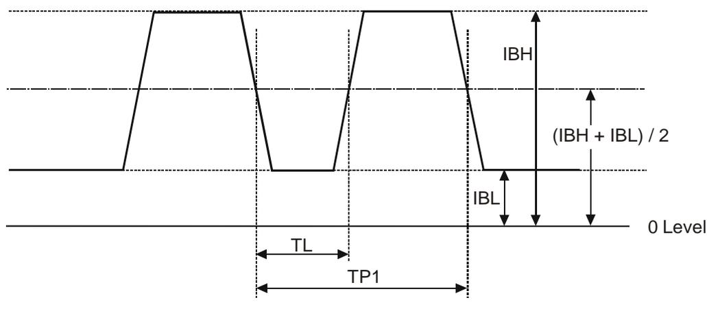
Figure L.3 - Read-out signal from NBCA
