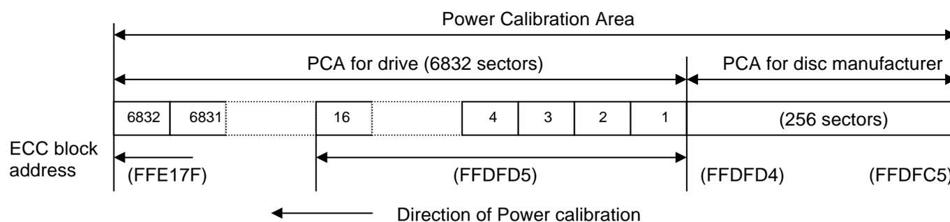
Figure 58 - Structure of the Power Calibration Area
