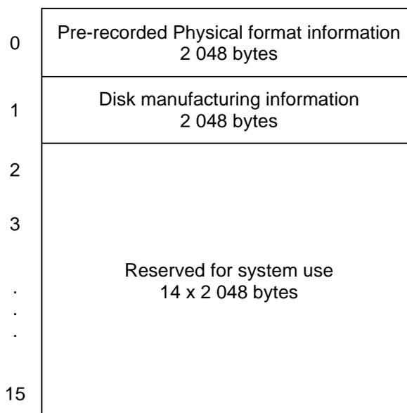
Figure 38 – Structure of a Control data block
