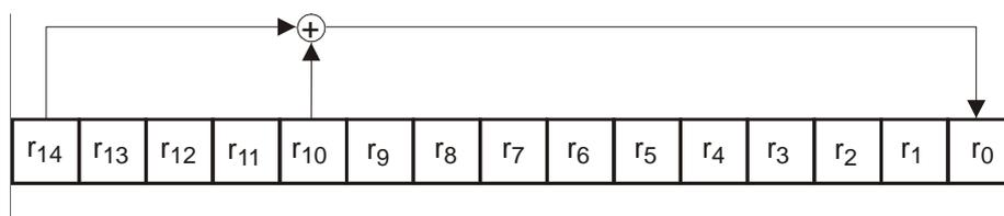
Figure 26 - Feedback shift register for generating scramble data
