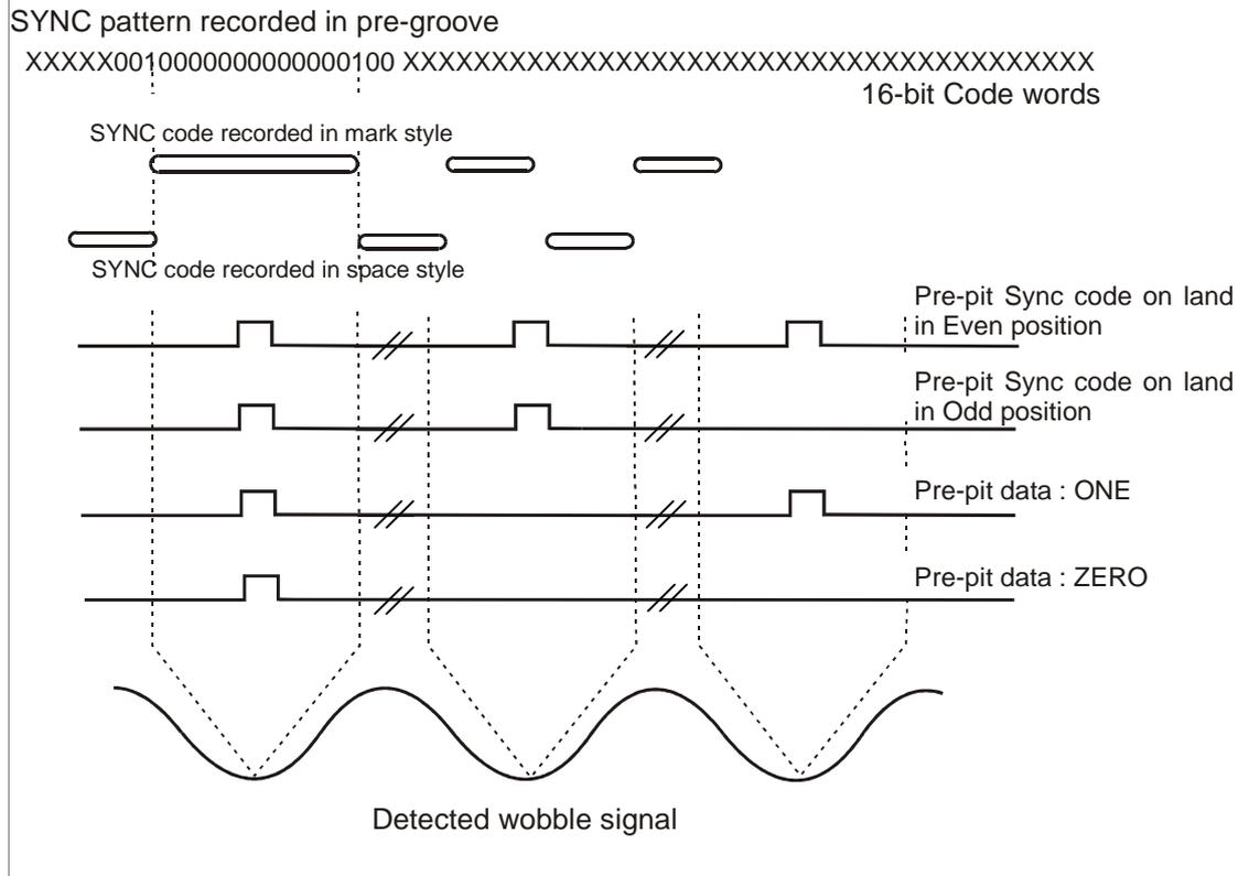
Figure 42 - Relationship of signals recorded in groove and land
