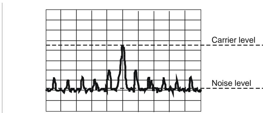
Figure 21 - Measurement of the wobble CNR
