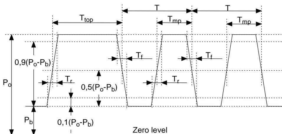
Figure 17 – Write pulse
