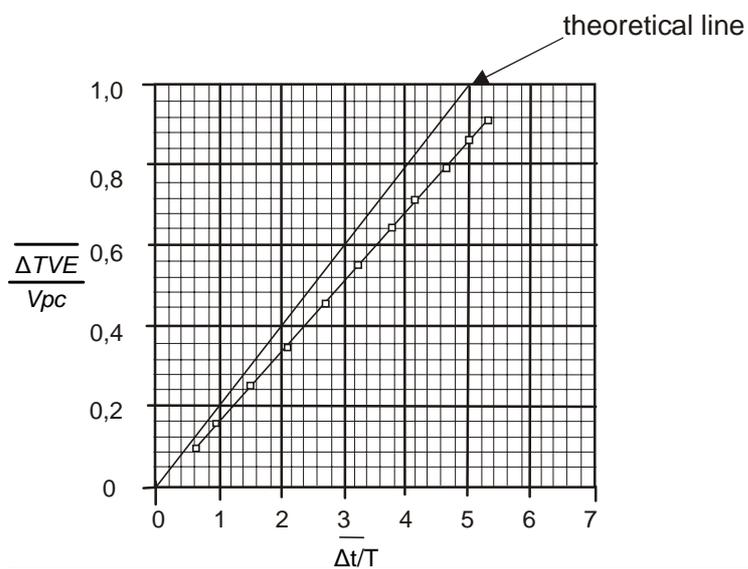
Figure C.3 -  $\overline{\Delta t/T}$  vs.  $\overline{\Delta TVE}/V_{pc}$
