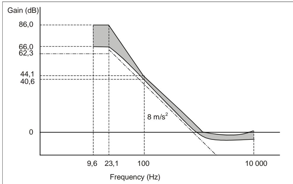
Figure 4 - Reference servo for axial tracking
