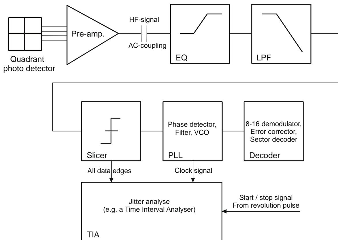
*Figure F.1 - General diagram for jitter measurement*
