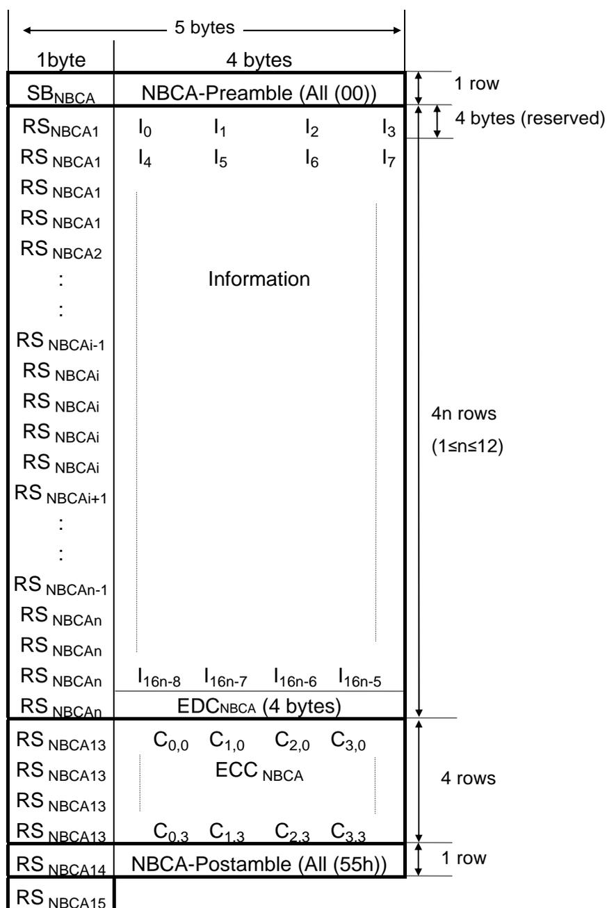
Figure L.2 - NBCA-Data structure
