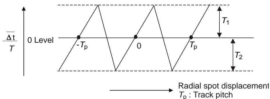
Figure 13 - Differential phase tracking error signal
