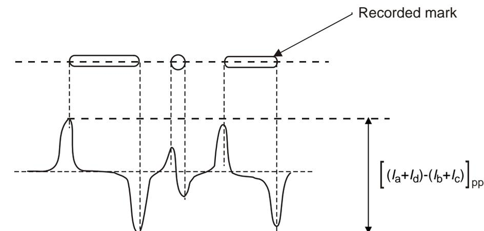
Figure 14 - Tangential push-pull signal
