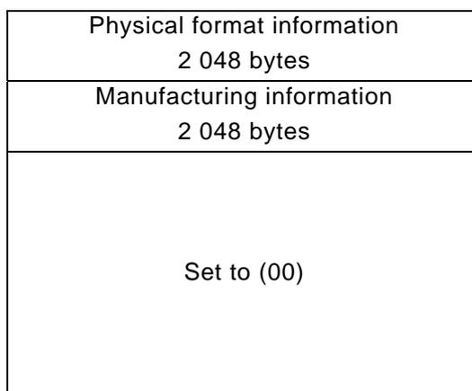
Figure 39 – Structure of Physical format information block
