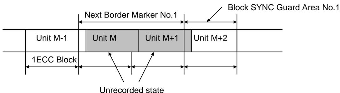
*Figure M.4 – Structure of Next Border Marker*
