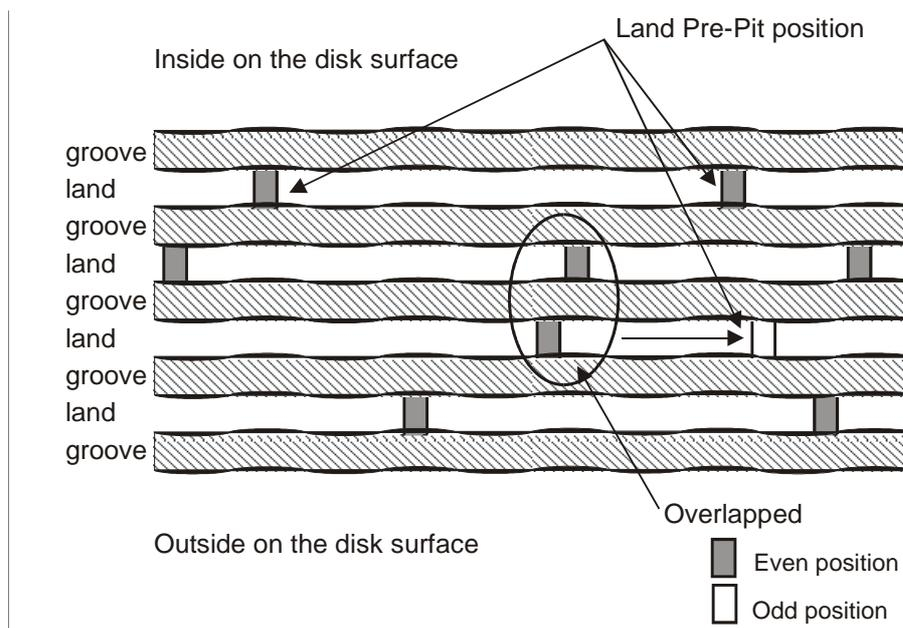
Figure 43 - Layout of land Pre-pit positioning
