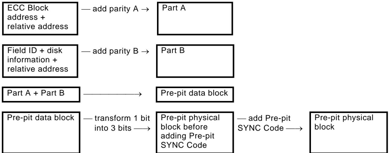
Figure 46 - Processing order to construct a Pre-pit block
