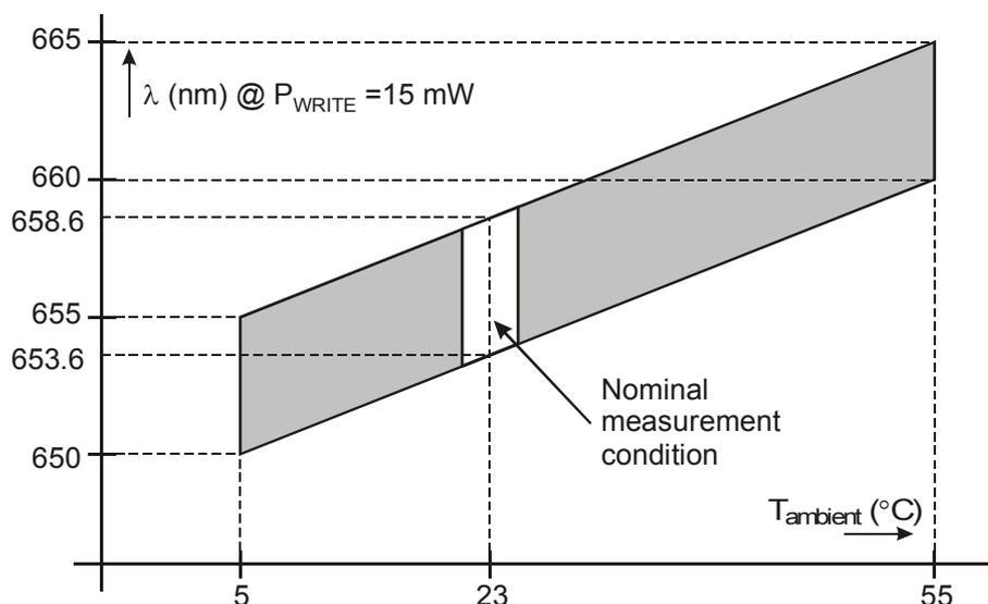
*Figure J.1 - Wavelength/Temperature diagram
