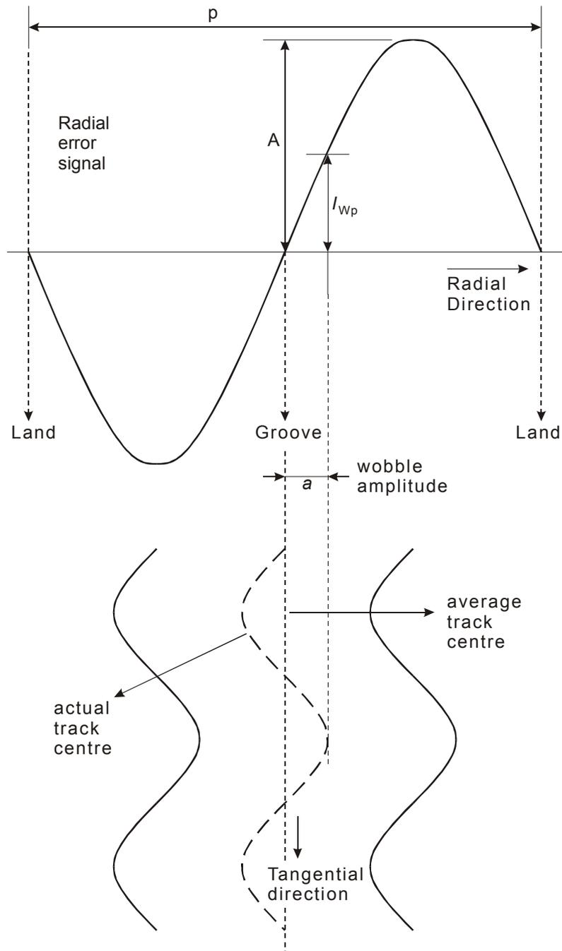
Figure M.1 - Wobble amplitude of the groove
