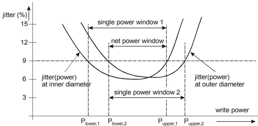
Figure 31 - Example of the write power windows
