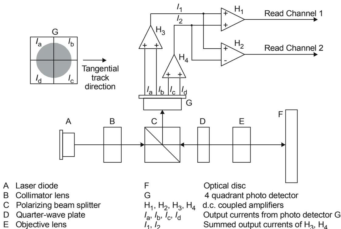
Figure 2 - Optical system of the Reference Drive
