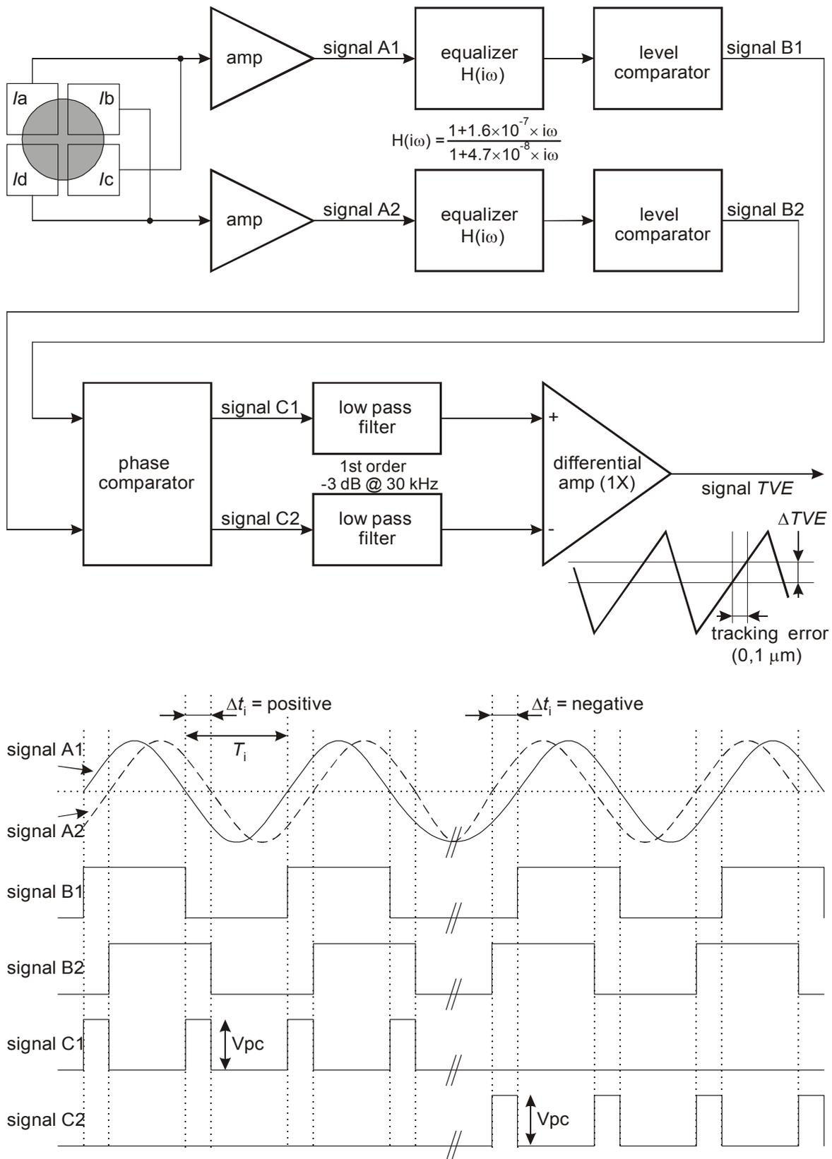
Figure E.1 - Circuit for tracking error measurements
