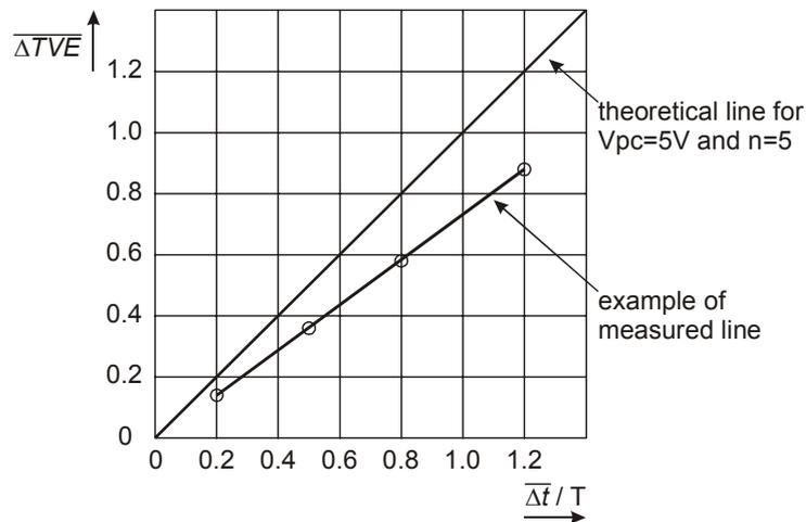
Figure E.3 -  $\overline{\Delta TVE}$  versus  $\overline{\Delta t/T}$
