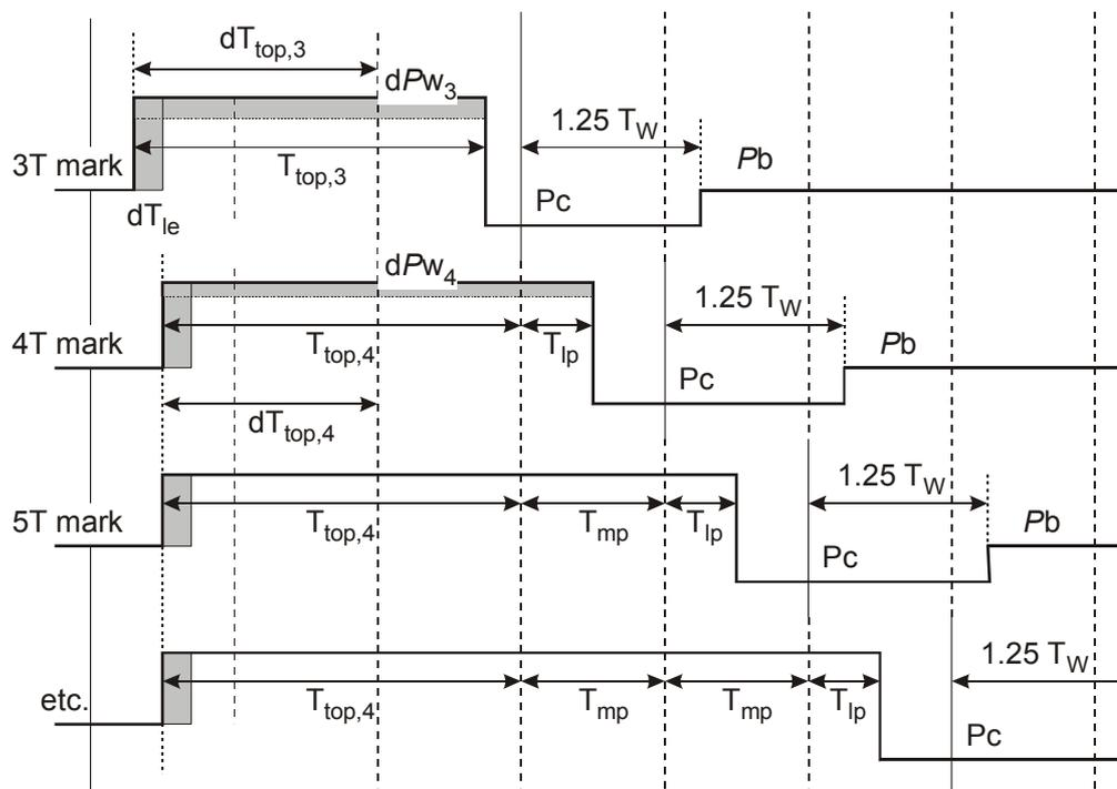
Figure F.4 - Examples of a "blocked" waveform
