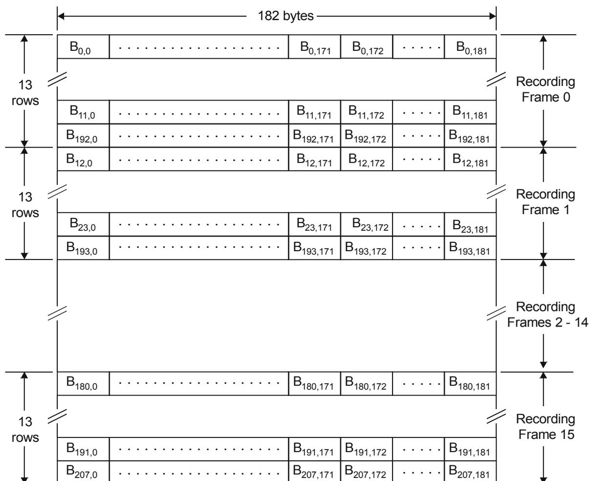
Figure 14 - Recording Frames obtained from an ECC Block
