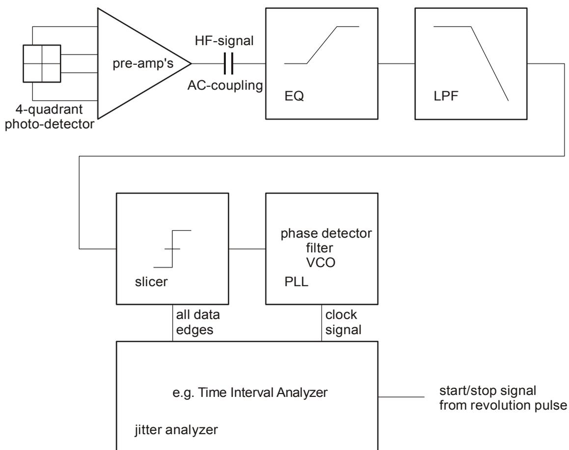
*Figure D.1 - General diagram for jitter measurement*
