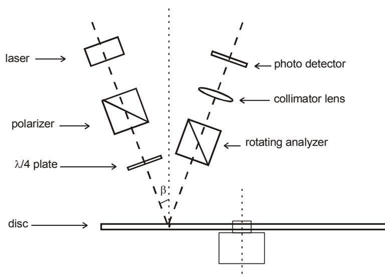
Figure C.2 - Example of a device for the measurement of birefringence
