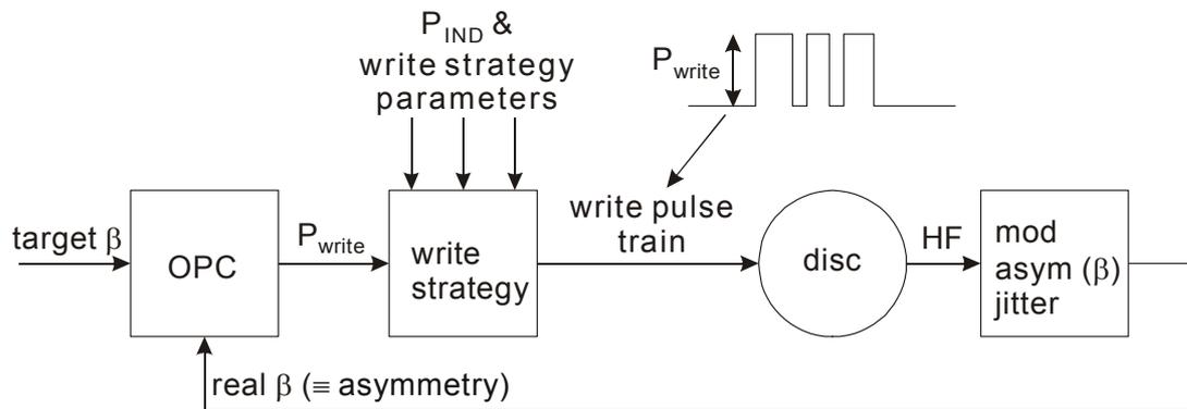
Figure H.1 - Schematic diagram of OPC procedure
