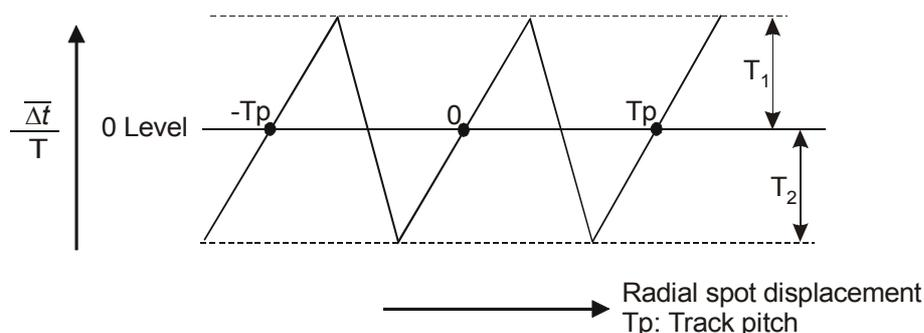
Figure 34 - Differential phase tracking error signal
