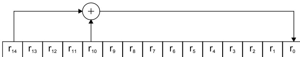
Figure 12 - Feedback shift register
