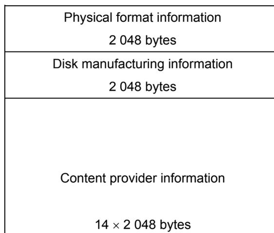
*Figure 24 — Structure of a Control Data Block*
