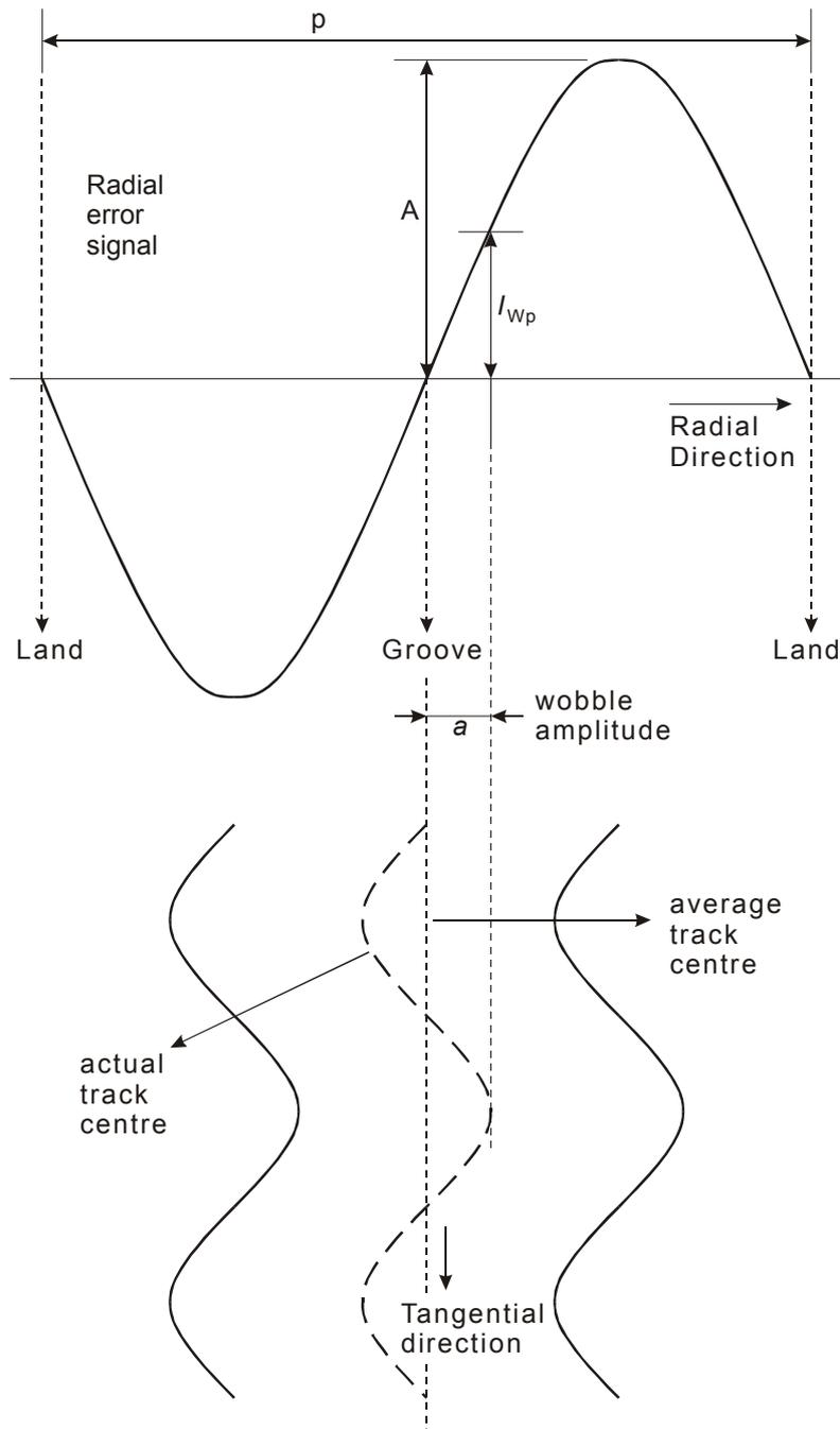
Figure K.1 — Wobble amplitude of the groove
