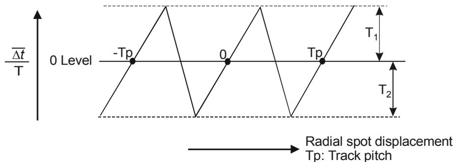
Figure 29 — Differential phase tracking error signal
