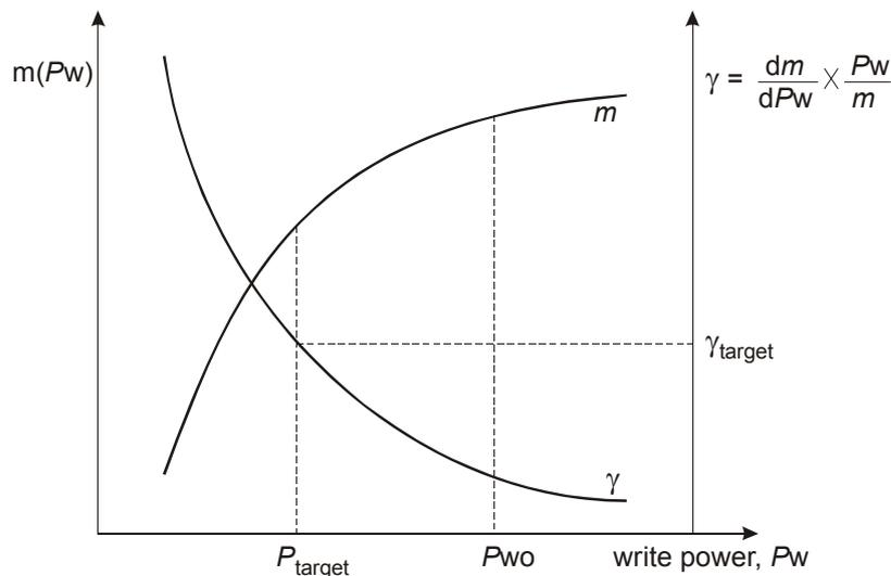
Figure I.1 — Modulation and Gamma functions versus power
