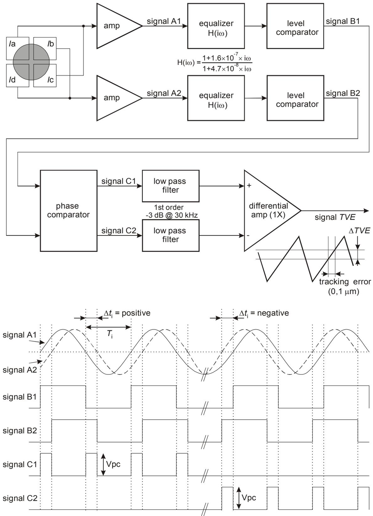
Figure F.1 — Circuit for tracking error measurements
