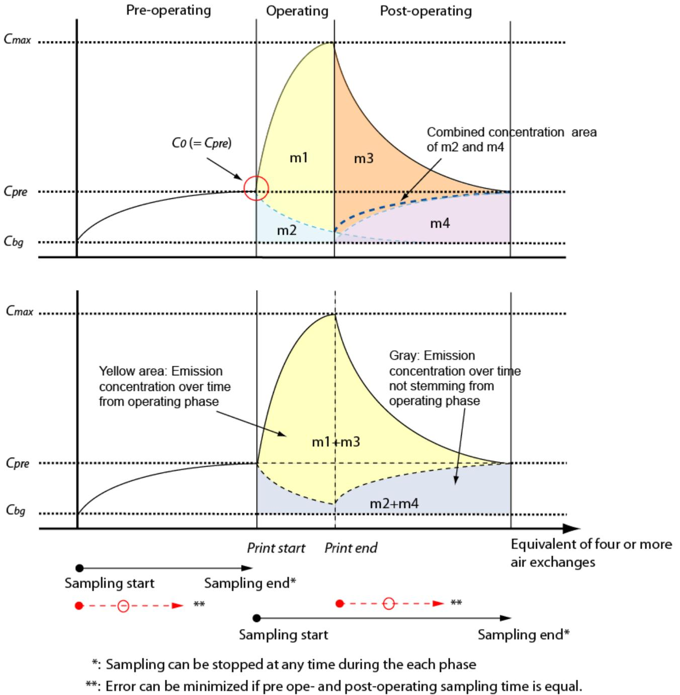
Figure C.1 — Representation of concentration change during printing and post operating phase
