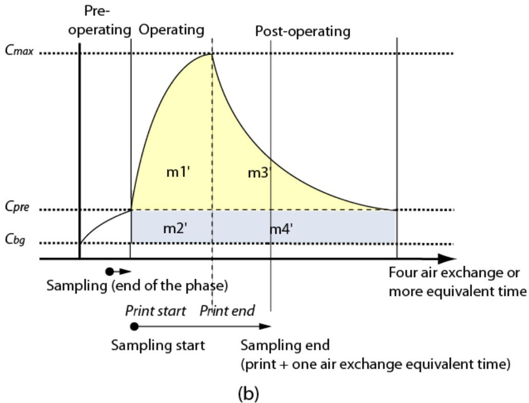
Figure C.2 — Model for equilibrium and constant  $C_o$  (a) and (b) RAL-UZ 171 Option model
