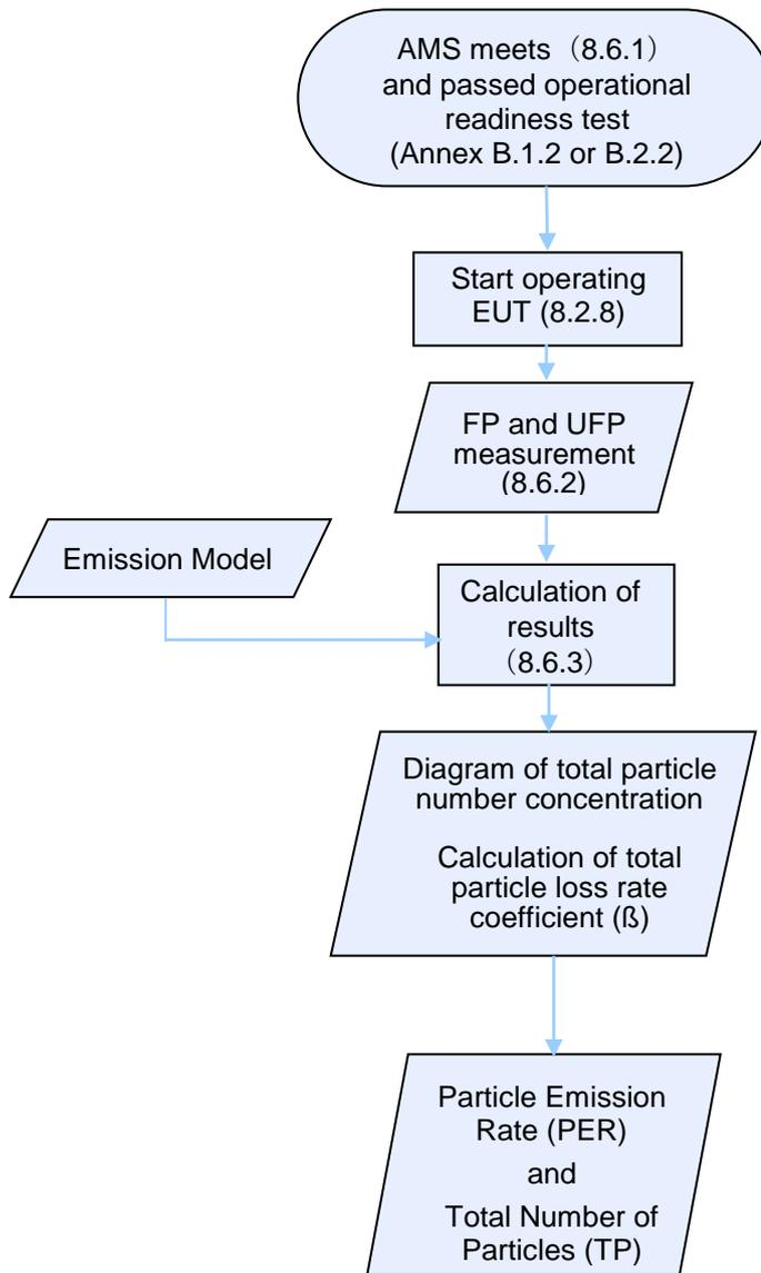
**Figure 5 — Determination method for FP and UFP emissions**
