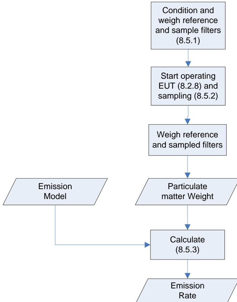
Figure 4 — Determination method for particulate matter
