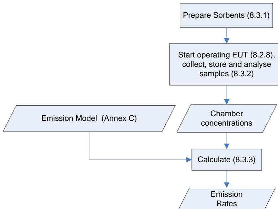
Figure 2 — Determination method for VOC, carbonyl compounds
